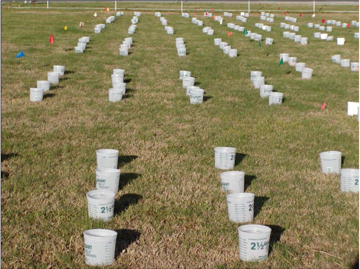
Figure 2-5. Catch-can display for uniformity tests on turfgrass plots.
