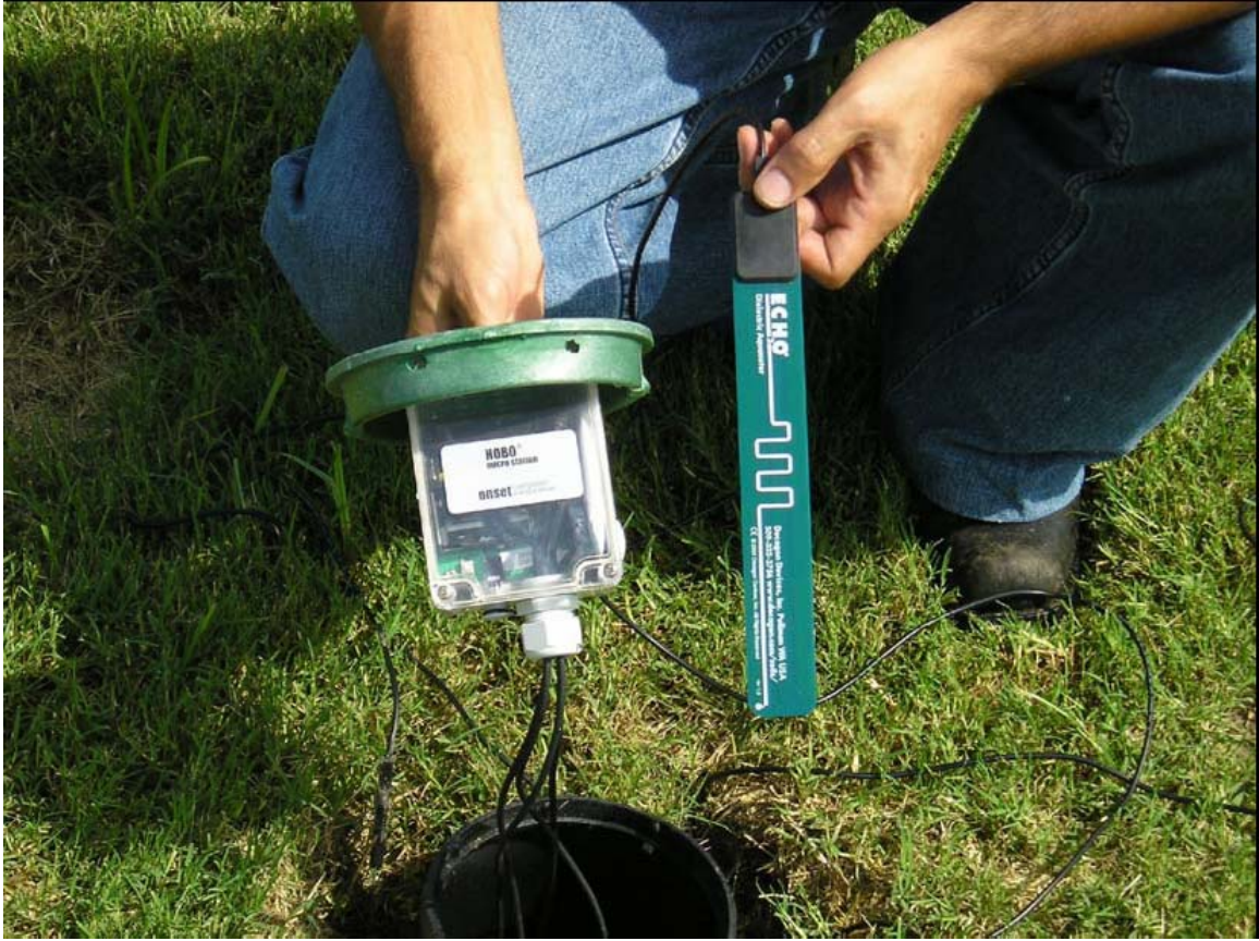
Figure 2-12. ECH 2 O probe, capacitance soil moisture probe shown with a HOBO data logger as installed for this study.
