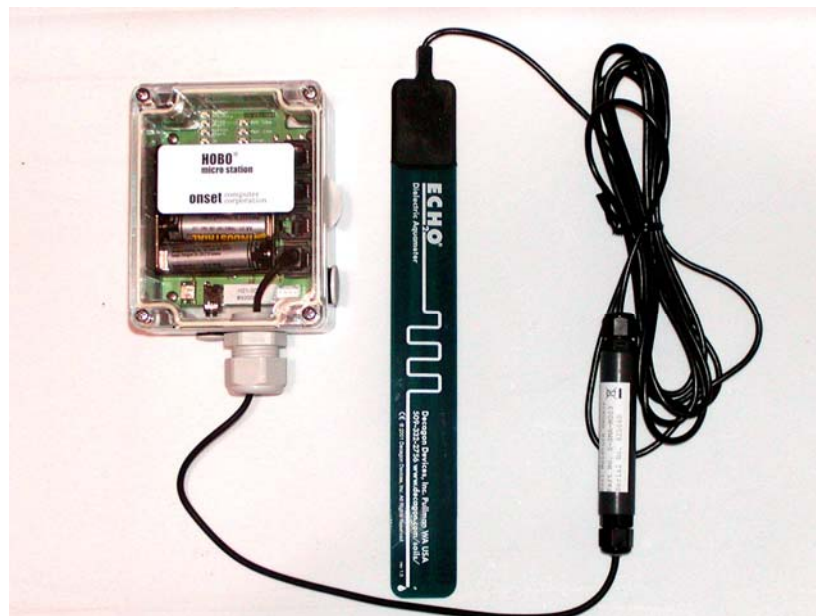
Figure 4-7. ECH 2 O probe hooked up to a HOBO Micro Station datalogger.
