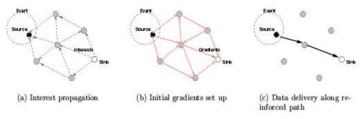
Figure 5. Schematic diagram for directed diffusion
