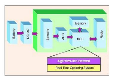
Figure 1. System architecture of a typical wireless sensor node
