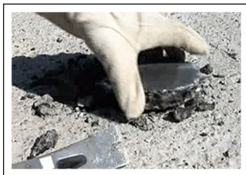
Figure 5.9. Removing sensor shell top
