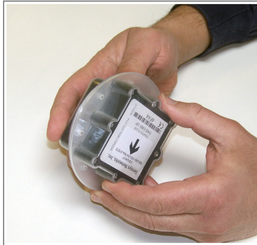
Figure 4.4. Fitting top of sensor shell to bottom of sensor shell
