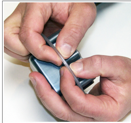
Figure 4.6. Pinching the shell edges together to seat the pins.
