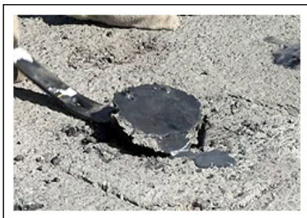
Figure 5.8. Removing sensor shell top
