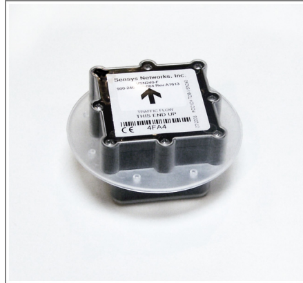
Figure 4.8. Finished sensor and shell assembly
