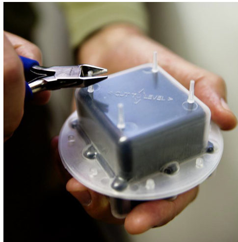
Figure 4.10. Trimming shell legs
