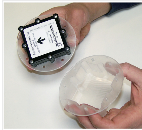
Figure 4.3. Placing sensor in shell
