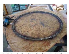
There's 24' of welding in each pulley and 97 segments that make the sidewalls of the big V pulleys.
