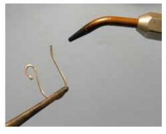
Then it occurred to me - I could melt the wire smooth. One quick touch in the flame of the propane/oxygen Little Torch does the trick - not enough to
