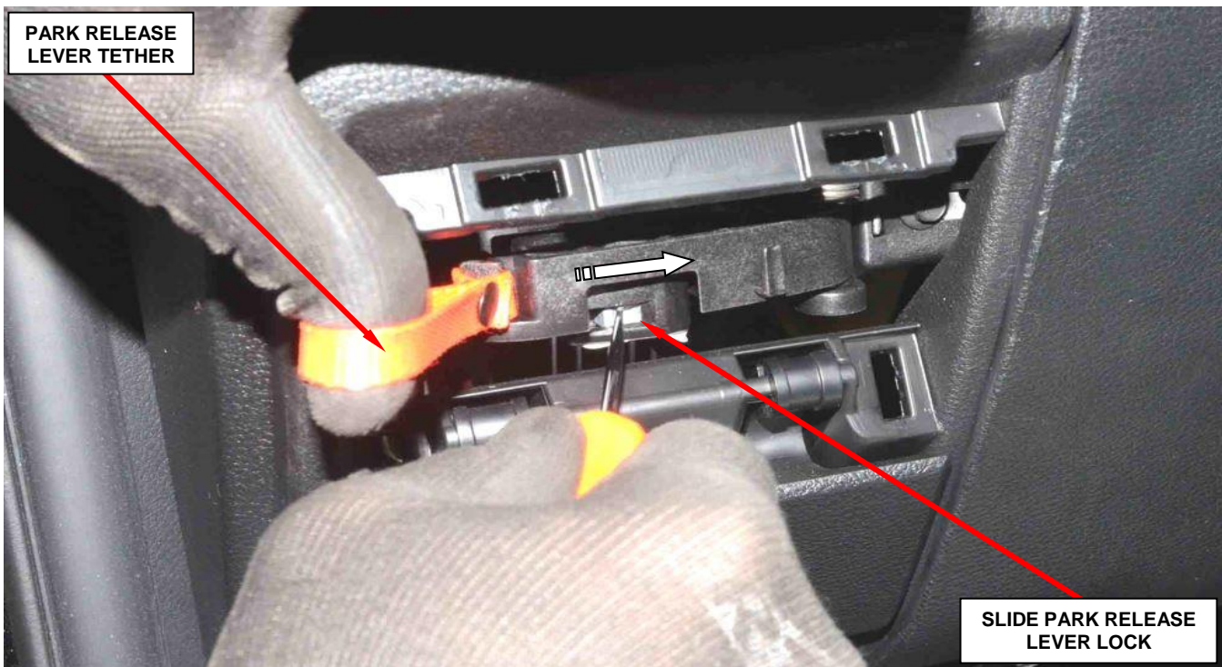
Figure 3 - Transmission Manual Park Release
