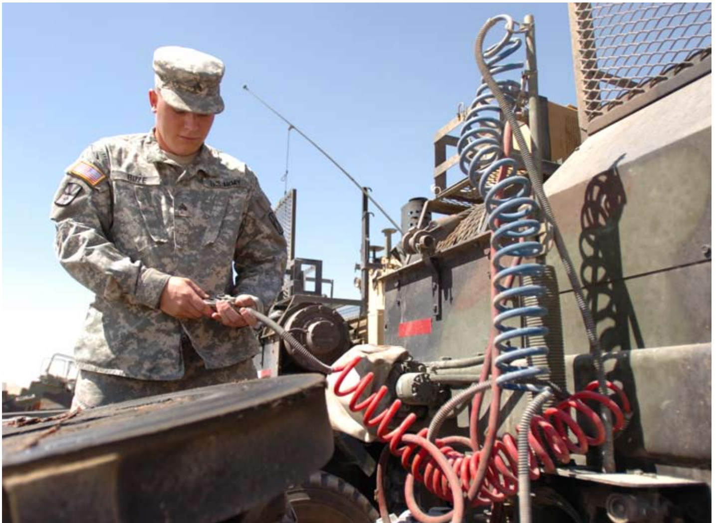
Spc. Raymond Boze checks the connections of an air line hose on a Heavy Equipment Transporter truck recently at Camp Arifjan, Kuwait. Boze has served 11 months of a 12-month deployment where he survived three separate IED attacks. Boze is a member of Battery B, 1/77 Field Artillery from Fort Sill Okla.
