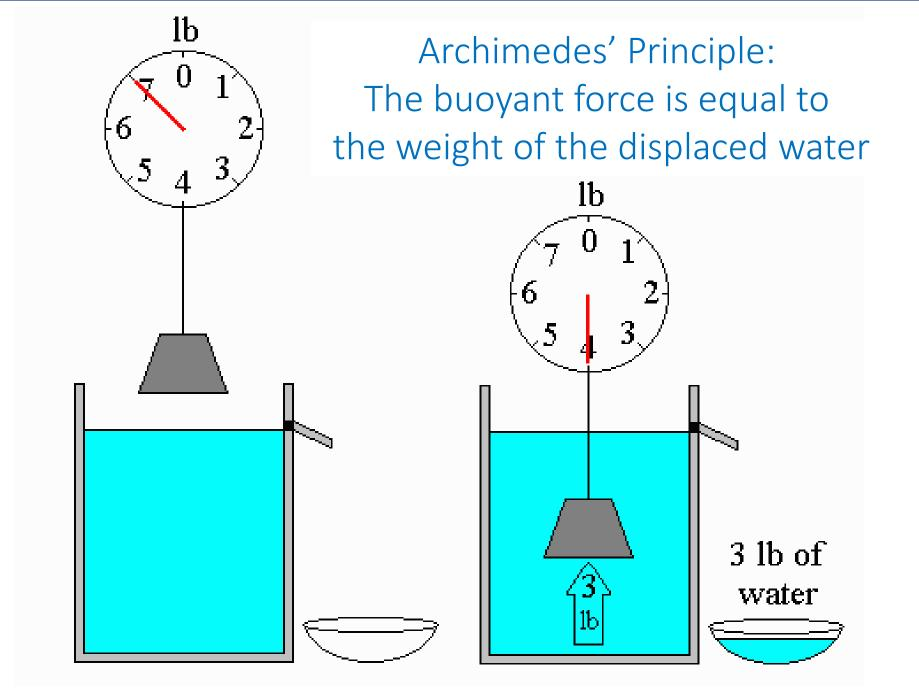
Archimedes' Principle: The buoyant force is equal to the weight of the displaced water
