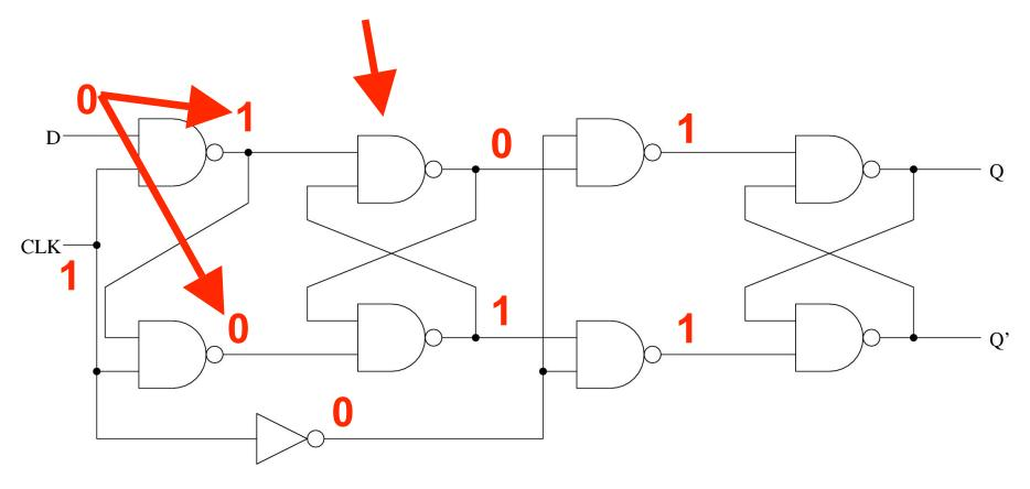
Clock transitions from high to low results in a 'reset' of the slave latch
