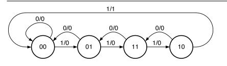
Figure 14.6: State diagram for finite-state machine of Table 14.2. The circles represent the four states. Each arrow represents a *state transition* from a current state to a next state and is labeled *input*/em output - the input that causes the transition, and the output in the current state for that input.
