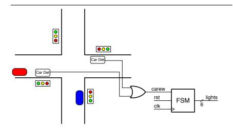
Figure 14.7: Controlling traffic lights at a road intersection with a FSM. Our FSM has two inputs, a reset (rst), and a signal that indicates that a car is waiting on the east-west road (carew). The FSM has six outputs that control the three north-south lights (green, yellow, red), and the three east-west lights.
