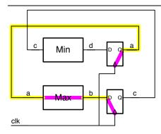
Figure 15.6: Setup-time constraint. The maximum path from the clock on a source flip-flop to the clock on a destination flip-flop is shaded. From the rising edge of the clock, the signal must propagate to the Q output of the flip-flop  $(t_{dCQ})$  and propagate through the maximum-delay logic path  $(t_{dab})$  at least a setup time  $(t_s)$  before the next clock edge. In this case the signal arrives slightly early  $(t_{slack})$ .
