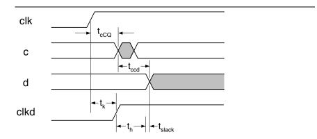
Figure 15.11: Timing diagram showing the effect of clock skew on the hold-time constraint.
