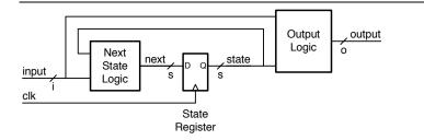
Figure 16.5: In general, a sequential datapath circuit consists of a state register, next-state logic, and output logic. The next-state and output modules are described by functions rather than tables.
