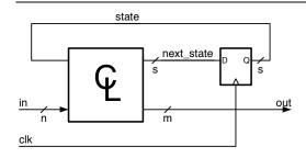
Figure 14.4: A *synchronous* sequential circuit breaks the state feedback loop with a clocked storage element (in this case a D-type flip-flop). The flip-flop ensures that all state variables change value at the same time - when the clock signal rises.
