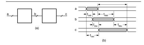
Figure 15.2: Propagation and contamination delay sum over a linear path. (a) Two modules in series with input a, intermediate signal b, and output c. (b) Timing diagram showing that  $t_{cac} = t_{cab} + t_{cbc}$  and similarly for propagation delay.
