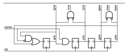
Figure 14.9: Implementation of the traffic light controller FSM using a one-hot state encoding. Four flip-flops are used, one corresponding to each state. The state transition arrows into a state directly translate into the logic preceding the corresponding flip-flop.
