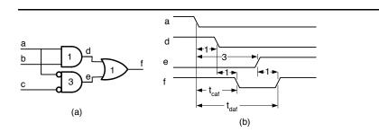
Figure 15.3: A circuit with a hazard illustrating propagation and contamination delay.
