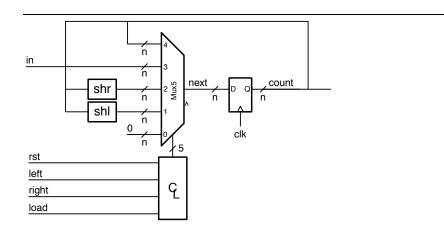
Figure 16.14: Block diagram of a left-right-load shift register.
