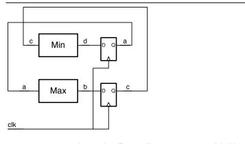
Figure 15.5: A simple FSM to illustrate setup and hold constraints
