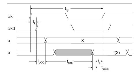
Figure 15.12: Timing diagram showing the effect of clock skew on the setup time constraint.
