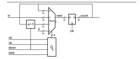
Figure 16.8: Block diagram of an up/down/load counter.
