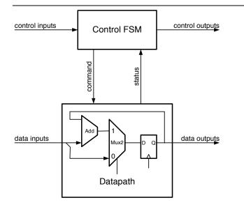
Figure 16.17: Systems are often partitioned into datapath, where the next state is determined by function units, and control, where the next state is determined by state tables.
