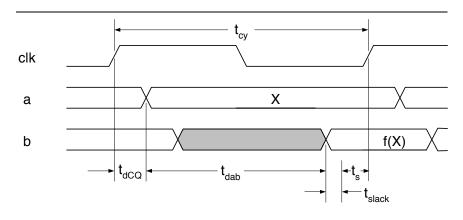
Figure 15.7: Timing diagram illustrating the setup-time constraint.
