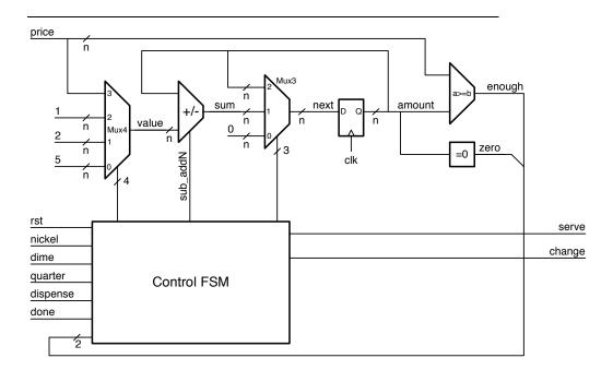
Figure 16.19: Block diagram of a vending machine controller.
