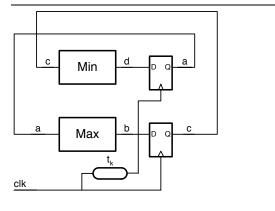
Figure 15.10: FSM of Figure 15.5 with clock skew.
