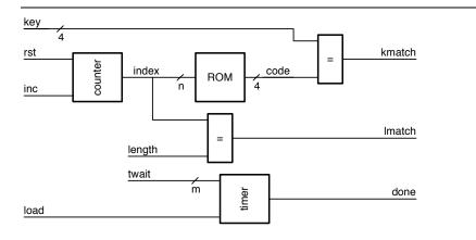
Figure 16.27: Block diagram of datapath portion of combination lock.
