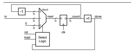
Figure 16.10: Block diagram of a timer FSM.
