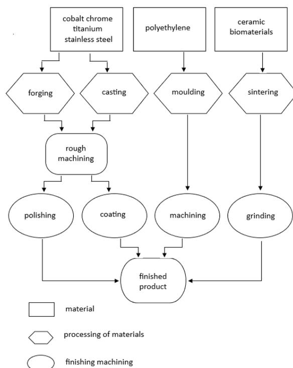
**Figure 2.** Manufacturing process of hip joint
