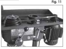
2. Lever the motor, on its bracket, away from the head, by turning lever B - Fig.11, anticlockwise so that tension is applied to the belts.
