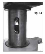
To disconnect the chuck from the arbour, give it a sharp tap with a soft head mallet to break the taper seal.
