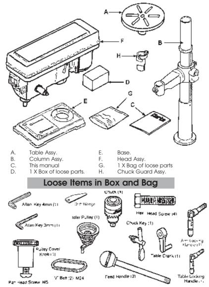
Check the parts against the above list and refer to the following diagrams. Should there be any deficiencies or damage, you should contact your CLARKE dealer immediately .
