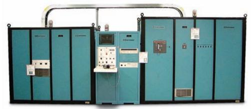
testing at high, low and nominal line voltages and all points in between. The Hipotronics units are capable of up to 2000 amps, 0-4160 volts and are equipped with Yokogawa Power Analyzers for power measurements. Independent control of each phase voltage allows for the introduction of a degree of phase imbalance to test "real world" conditions. The system's PC monitors the Hipotronics settings and test conditions and logs test data.
