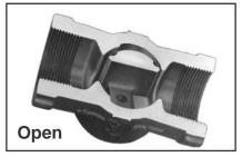
**KEY PORT VALVE** eccentric action and resilient seating assure lasting dead-tight shutoff. As the eccentric plug rotates 90 degrees from open to closed, it moves into a raised eccentric seat.
