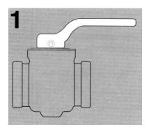
FIG 483 lever - Order as a separate item by giving "FIG 483" followed by valve size code (0100 = 1", 0200 = 2", etc.). Note: FIG 487 Memory Stop cannot be used with the FIG 483 lever.
