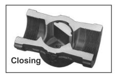
As the plug closes, it moves toward the seat without scraping the seat or body walls so there is no plug binding or wear. Flow is still straight through making the throttling characteristic of this valve ideal for manual throttling of gasses and liquids.
