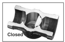
In the closed position, the plug makes contact with the seat. The resilient plug seal is pressed firmly into the seat for dead-tight shutoff. Eccentric plug and seat design assure lasting shutoff because the plug continues to move into the seat until firm contact and seal is made.
