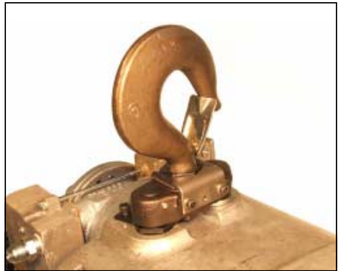
Figure 7-16. View of Upper Hook Assembled to Hoist Frame (Double Reeved Models)
