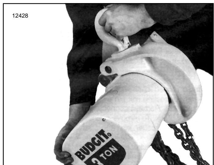
Figure 7-2. Removing 3 Ton Hanger Bracket from Hoist Frame
