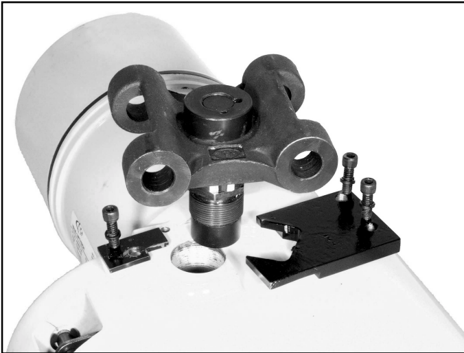
Figure 7-17. Removing Suspension Lug (1/4 through 1 Ton Models)
