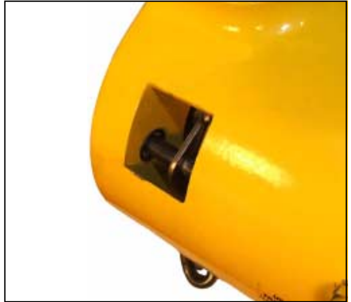
Figure 7-12. Removing Chain Guide Support Pins
