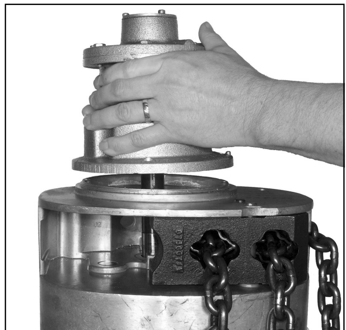
Figure 7-8. Removing Motor Assembly
