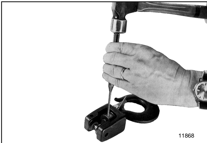
Figure 7-23. Removing Roll Pin Securing Hook Nut to Hook Shank
