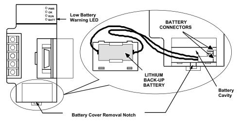
Figure 6-1. Backup Battery for RAM Memory
