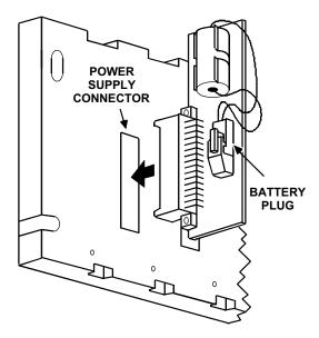
Figure 6-2. Installing the Battery Accessory Kit
