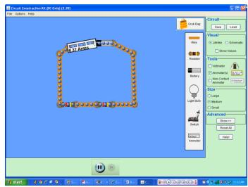
The second series circuit will have a 12  $\Omega$  and a 24  $\Omega$  resistor in it.
