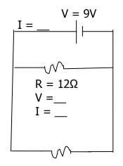
R = 24Ω V = \_\_\_ I = \_\_\_ Make a second parallel circuit with a 12  $\Omega$  and a 24 $\Omega$  resistor. Record the voltages and currents through each part.
