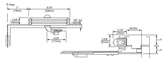
Mounting holes for closer body are spaced 3/4" (19mm) vertically x 9-1/16" (230mm) horizontally.
