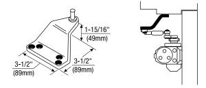
Extra-Clearance - #2018S Offset Soffit Plate: For use where the need for additional clearance prevents use of the standard soffit plate. This plate mounts to the frame soffit to provide up to 2" (51mm) of clearance when a separate overhead door holder is used. Standard mounting requires a 2-5/8" (67mm) wide frame soffit. It may also be used where unusually high frame stops or weatherstripping prevents the use of other soffit plates.
