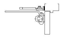
Converting Old Hold Open Installations - #2017 Adapter Plate: For use on old hold open installations with 2-1/2" (64mm) hole spacing on the holder bracket. Plate uses existing holes in either door or frame and accepts the new hold open bracket with 1-3/4" (44mm) hole spacing. For regular arm or top jamb installations.
