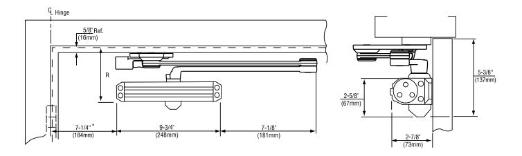
Mounting holes for closer body are spaced 3/4" (19mm) vertically x 9-1/16" (230mm) horizontally.
