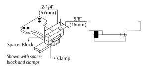
**Wide Frame - #6191 Reinforcing Kit:** Optional for use with all parallel arm Unitrol Door Controls. Used to support the soffit plate on installations with deep frames. Clamps may be used with or without the spacer block, depending on frame conditions.
