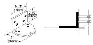
**Flush Rabbeted Transom - #2019L Angle Bracket:** For use where flush transom conditions prevent mounting of the standard soffit plate. This bracket is used in combination with the arm's soffit plate.
