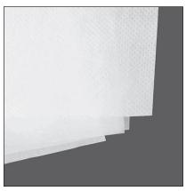
A multi-ply laminate is used with our sub and one micron absolute grades for longer life and greater solids removal.
