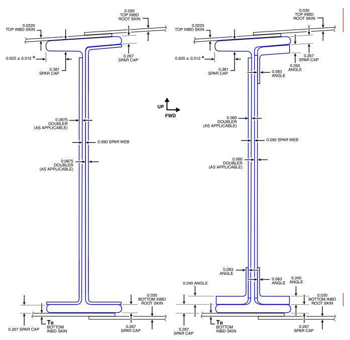
NOTE: The minimum allowable dimensions are shown in View A-A and B-B,
