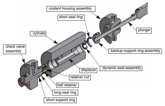
Figure 7-41: High-pressure Wet-end Assembly
