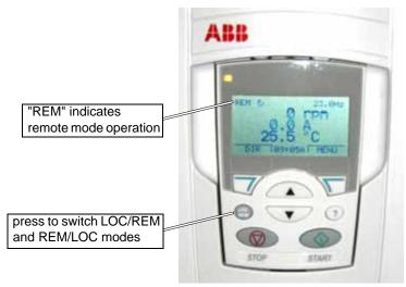
Figure 5-8: VFD Remote (REM) Mode
