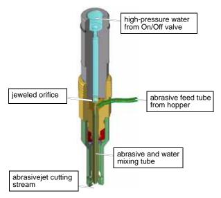
Figure 2-23: Internal Workings of the Abrasivejet Nozzle
