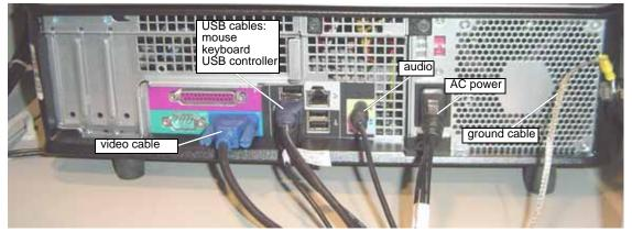
Figure 2-17: PC Rear Panel Cable Connections
