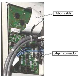
Figure 5-11: Keypad Ribbon Cable and 34-Pin Connector Location
