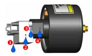
Figure 4-4: Sources of Water Leaks in the On/Off Valve
