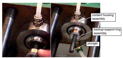
Figure 7-44: Sliding the Backup-support Ring Assembly onto the Plunger
