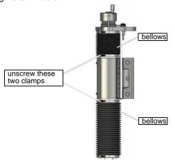
Figure 6-12: Z-axis Assembly
