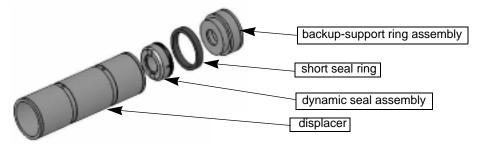
Figure 7-10: Sealing Assembly Components
