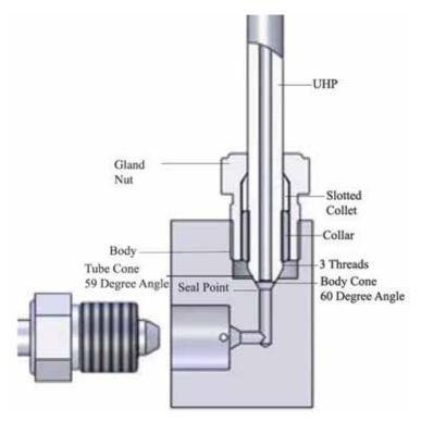
Figure 4-2: Components of the Ultra High-pressure Fitting
