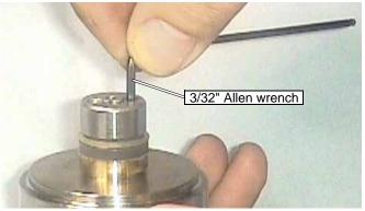
Figure 7-26: Tightening the Socket Head Screws
