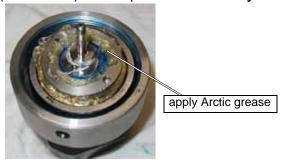
Figure B-24: Apply Arctic Grease to Top of Bearing Assembly
