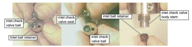
Figure 7-28: Inserting the Check Valve Ball and Check Valve Seat into the Inlet Ball Retainer
