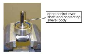
Figure B-14: Center the Socket Over the Surface of the Swivel Body
