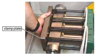
Figure 7-4: Clamp Plate Removal
