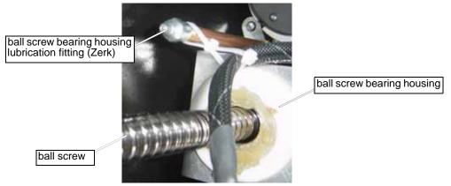
Figure 6-19: Grease Fitting for Lubricating the X-axis Ball Screw Bearing Housing
