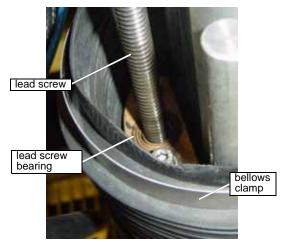
Figure 6-16: Motorized Z Lead Screw Bearing Location
