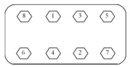
Figure 7-48: Clamp Plate Torque Sequence for Clamp Plate Nuts
