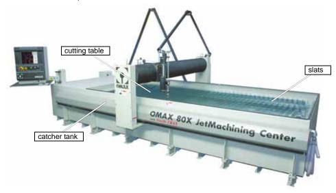
Figure 2-25: JetMachining Center Catcher Tank
