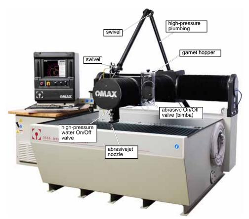
Figure 2-21: JetMachining Center Abrasive jet System Components (5555 illustrated)
