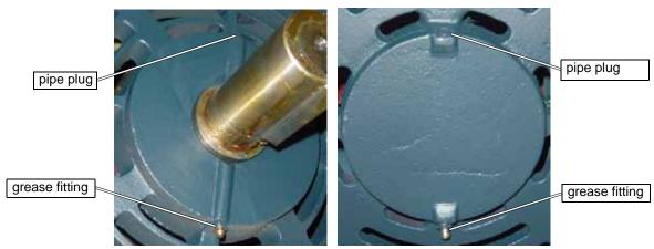
Figure 7-57: Location of Front and Rear Motor Grease Fittings and Pipe Plugs
