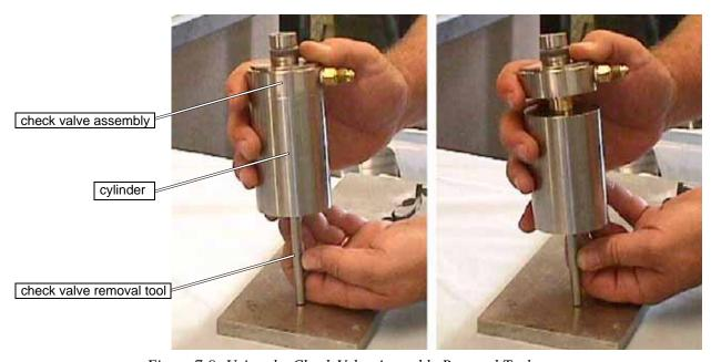
Figure 7-9: Using the Check Valve Assembly Removal Tool
