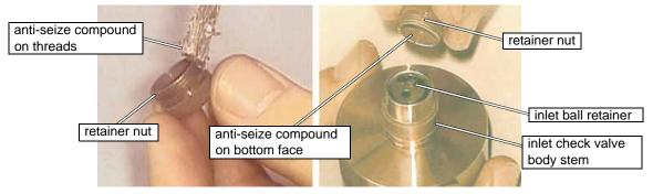
Figure 7-29: Applying Anti-seize Compound to Threads and Bottom Face of Retainer Nut
