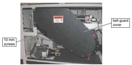
Figure 7-55: OMAX Pump Belt Guard Cover
