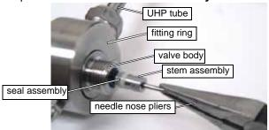
Figure C-8: Removing the Stem Assembly from the Valve Body
