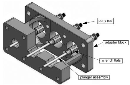
Figure 7-38: Adapter Block, Pony Rod and Plunger Assembly
