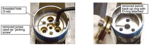
Figure B-8: Remove the Swivel Back-up Ring from the Swivel Assembly
