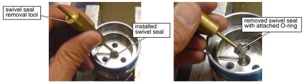
Figure B-9: Use the Removal Tool to Take Out the Swivel Seal and O-ring
