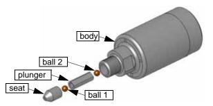
Figure 5-2: Safety Valve Internal Components
