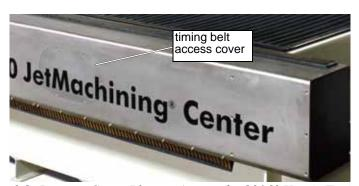
Figure 6-8: Remove Cover Plate to Access the 80160 X-axis Timing Belt
