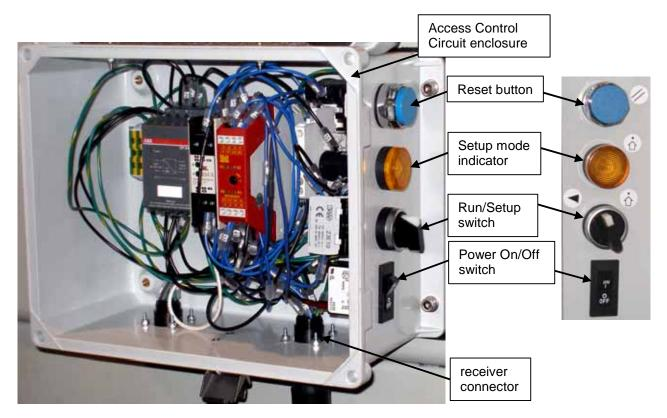
Figure A-2: Access Control Enclosure Attached to Side of OMAX Controller
