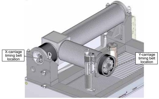
Figure 6-3: Timing Belt Locations Typical of OMAX Cantilever Tables
