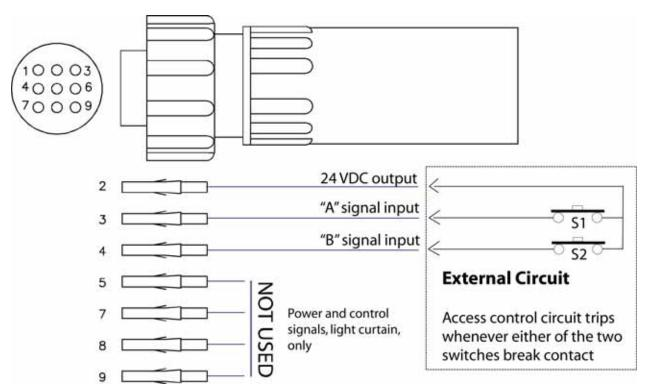
Figure A-1: External Electrical Circuit Requirement for the ACC
