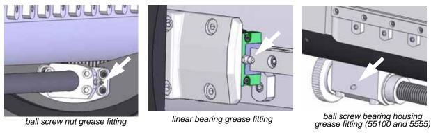
Figure 6-11: Lubrication Fittings for Cantilever Style X, Y Carriages
