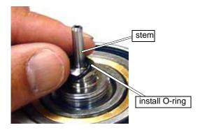
*Figure B-21: Replace the O-ring on the Swivel Body*
