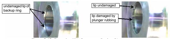
Figure 7-17: Example of Lip Damage to Backup Ring
