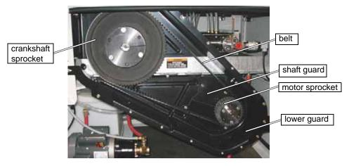
Figure 7-56: OMAX Pump Belt with Belt Guard Cover Removed
