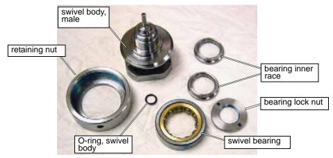
Figure B-17: Male Swivel Body Bearing Components
