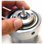
Figure B-22: Hand Tighten the Bearing Lock Nut
