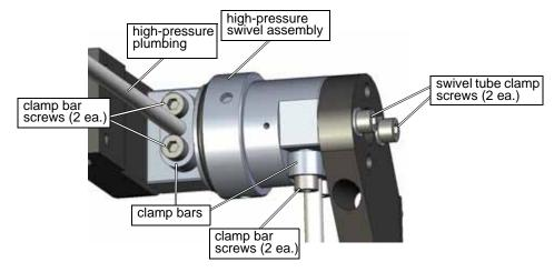
Figure B-2: Typical High Pressure Swivel Installation
