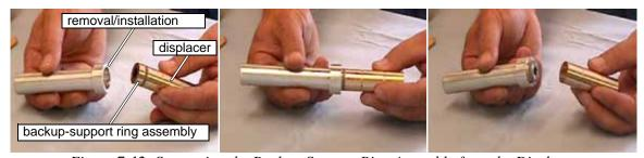
Figure 7-12: Separating the Backup-Support Ring Assembly from the Displacer.
