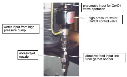
Figure 2-22: Components of an OMAX Abrasivejet Nozzle Assembly
