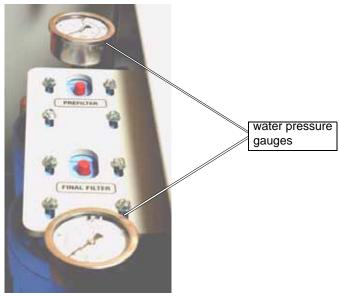
Figure 5-4: Pressure Gauges for Water Filters
