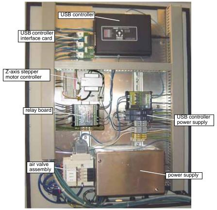
Figure 2-13: Controller Rear Door Internal Components
