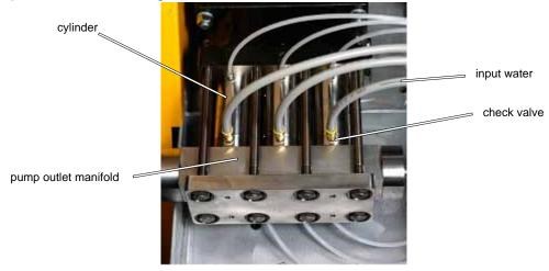
Figure 3-10: The High-pressure Wet-end of the OMAX Pump.
