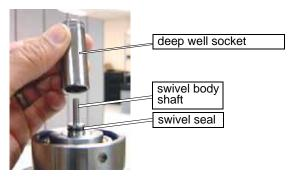
Figure B-13: Place a Deep Socket over the Swivel Body Shaft
