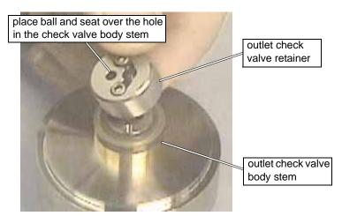
Figure 7-25: Placing the Outlet Check Valve Retainer on the Check Valve Body Stem
