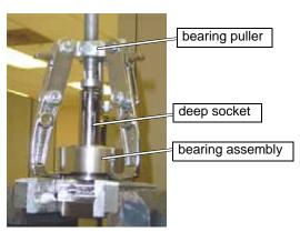
Figure B-15: Use the Bearing Puller to Remove the Bearing Assembly
