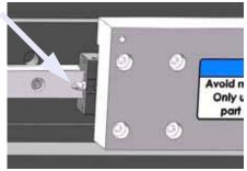
Figure 6-20: Grease Fitting for Lubricating the 2nd X-axis Linear Bearing
