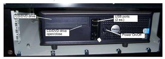
Figure 2-16: User Components on Front Panel of Controller PC
