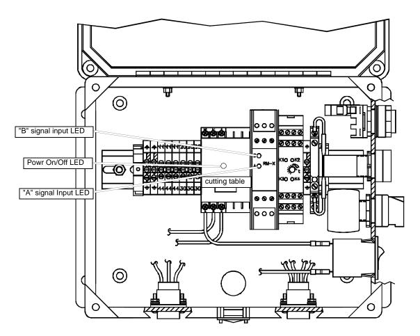
Figure A-3: ACC Status LEDs
