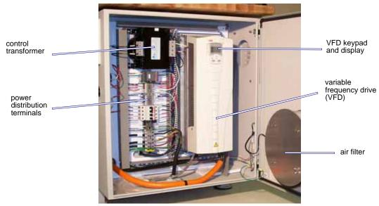
Figure 3-6: Pump Internal Components on Right Side
