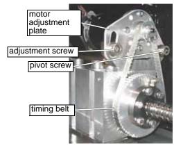
Figure 6-9: View of 80160 Timing Belt With Access Plate Removed
