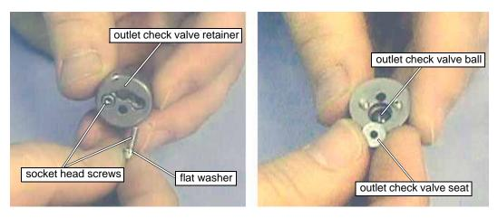
Figure 7-24: Inserting the Socket Head Screws
