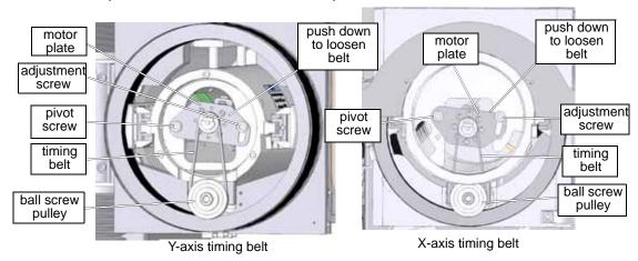
Figure 6-5: Components Involved in Adjusting the Timing Belt Tension
