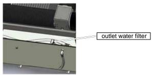
Figure 6-1: Outlet Water Filter Screen at Back of Tank
