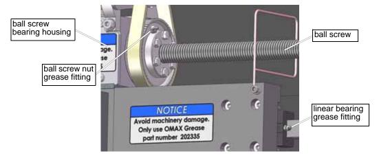
Figure 6-18: Grease Fittings for the 80160 Ball Screw Bearing Housing and Linear Bearing
