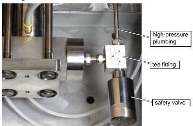
Figure 5-1: OMAX Pump High-pressure Safety Valve
