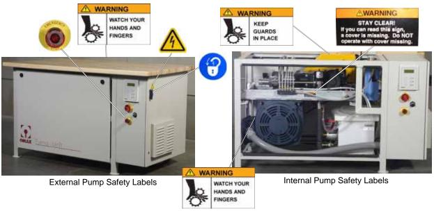
Figure 1-5: Safety Labels OMAX Pumps
