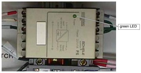
Figure 5-9: 24 VDC Power Supply
