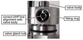
Figure C-17: Align the UHP Line with the Opening in the Fitting Ring
