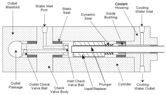
Figure 3-11: Details of the Pump Wet-end
