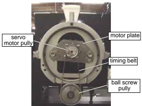
Figure 6-2: Example of Typical OMAX Servo Motor/Ball Screw Timing Belt Connection
