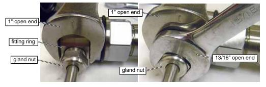
Figure C-4: Loosening the Valve Gland Nut using Two Open End Wrenches
