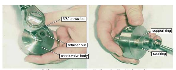
Figure 7-20: Removing the Retainer Nut from the Check Valve Body
