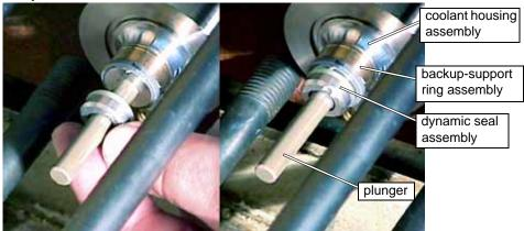
Figure 7-45: Sliding the Dynamic Seal Assembly onto the Plunger
