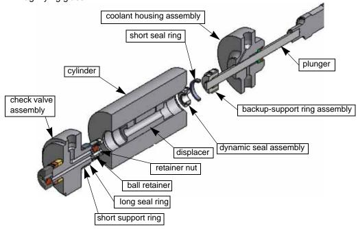
Figure 7-7: High-Pressure Wet-end Assembly Components
