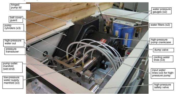
Figure 3-5: Top View of Pump with Lid Open
