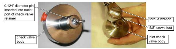
Figure 7-30: Installing the Inlet Retainer Nut
