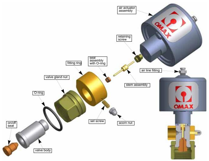
Figure C-6: Components of the OMAX Dual On/Off Valve
