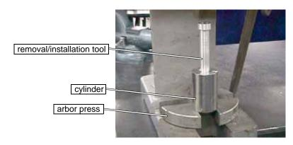
Figure 7-11: Removing the Sealing Assembly using an Arbor Press
