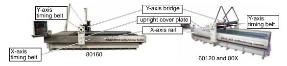
Figure 6-7: Timing Belt Locations for Bridge-style Tables
