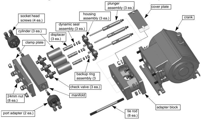
Figure 7-1: Major Components of the Wet-end Pump Assembly
