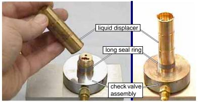
Figure 7-33: Installing the Liquid Displacer on the Check Valve Assembly
