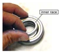
Figure B-19: Reinstalling the Bearing Inner Race
