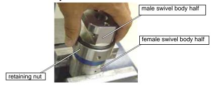
Figure B-25: Assemble the Two Swivel Body Halves
