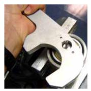
Figure B-23: Fully Tighten the Bearing Lock Nut using the Swivel Spanner Wrench
