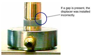
Figure 7-34: Reversed Displacer Example
