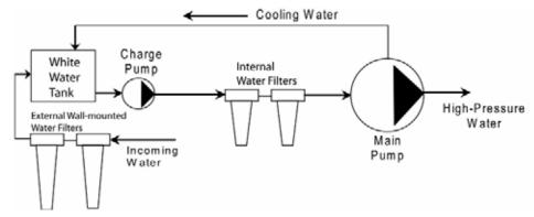
Figure 7-49: The Low-pressure Water Filtration System
