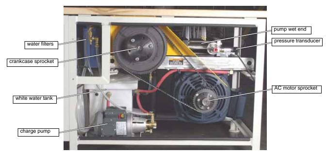
Figure 3-4: Pump with Rear Panel Removed
