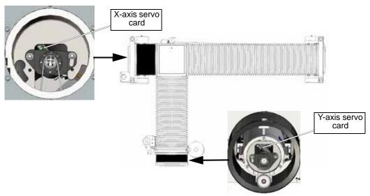
Figure 4-6: Servo Card Locations for Y- and X-axis 2626, 2626/xp, 2652, 5555, 55100 Servo Motors
