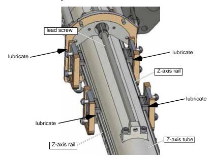
Figure 6-14: Z-axis Bearing Locations Requiring Lubrication
