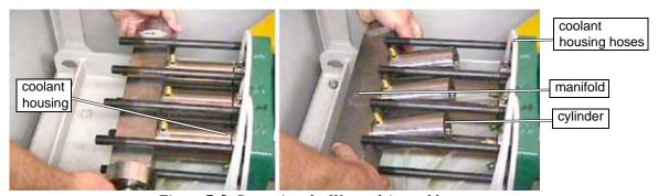
Figure 7-5: Removing the Wet-end Assembly
