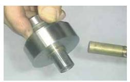
Figure 7-21: Using a Propane Torch to Remove the Support Ring
