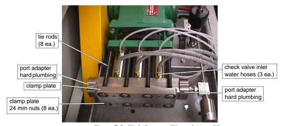
Figure 7-2: High-Pressure Wet-end Assembly
