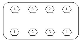
Figure 7-3: Nut Loosening Sequence for Removing Clamp Plate from High Pressure Assembly.
