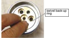
Figure B-11: Insert the Swivel Back-up Ring with a New O-ring Installed into the Swivel Body
