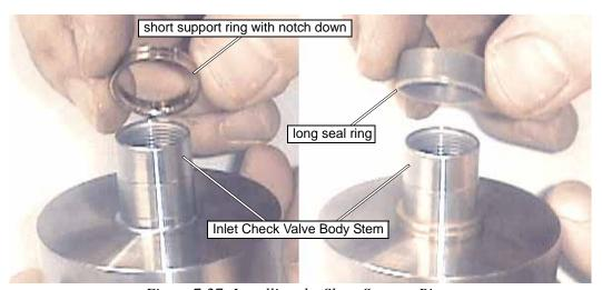
Figure 7-27: Installing the Short Support Ring
