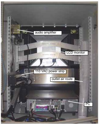
Figure 2-14: Controller Cabinet Internal Components
