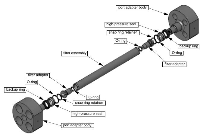
Figure 7-31: Port Adapter and Filter Assembly Components
