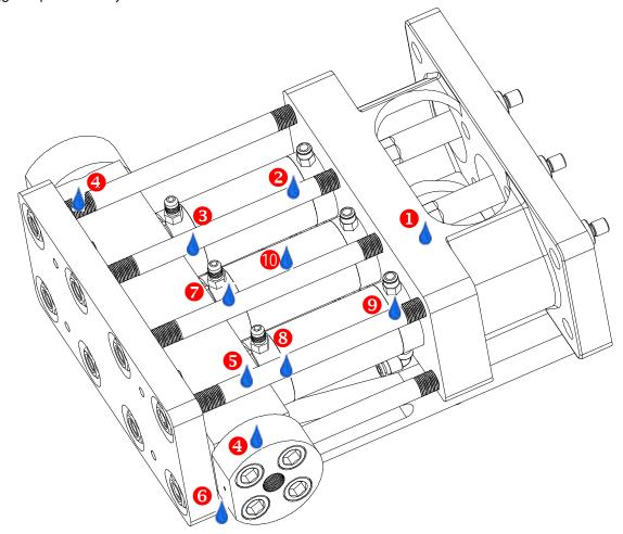
Figure 5-5: Sources of Water Leaks in the Wet-end Assembly
