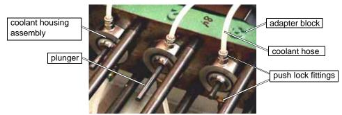
Figure 7-37: Removing the Coolant Housing Assemblies
