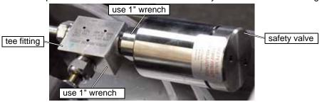
Figure 5-3: Safety Valve Removal
