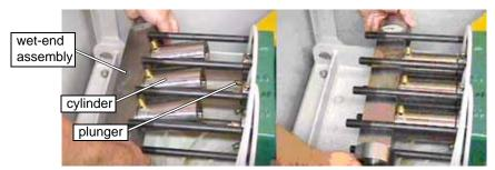
Figure 7-46: Sliding the Wet-end Assembly over the Plungers
