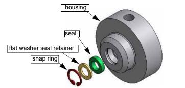
Figure 7-36: Coolant Housing Assembly Components
