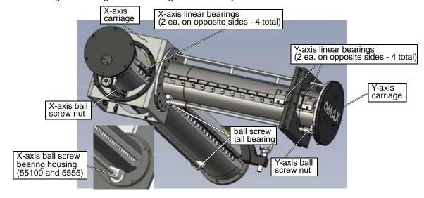
Figure 6-10: Lubrication Points on OMAX Cantilever Style X, Y Carriages
