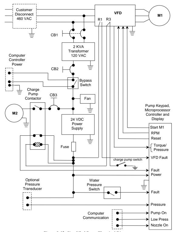
Figure 3-12: Simplified Pump Electrical Diagram
