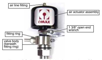
Figure C-2: Removing the Air Actuator Assembly
