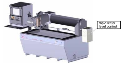
Figure 2-26: OMAX's Rapid Water Level Control
