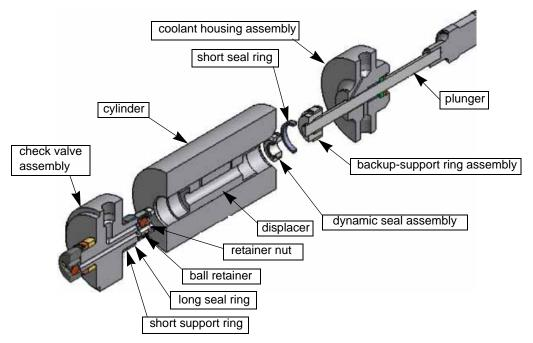
Figure 7-32: High-pressure Wet-end Assembly Components
