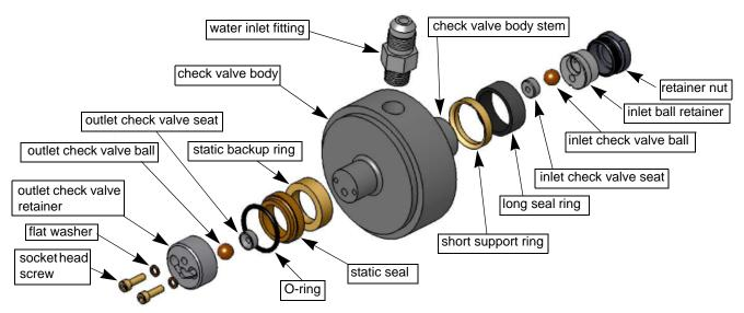
Figure 7-23: Check Valve Assembly Components
