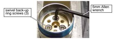
Figure B-12: Tighten the Three Screws to the Swivel Back-up Ring
