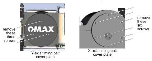
Figure 6-4: Carriage End Cover Screws Removed to Access Timing Belt
