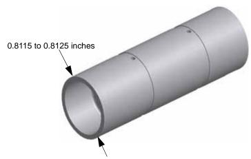
Figure 7-18: Liquid Displacer Measurements
