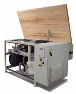
Figure 3-1: OMAX High-Pressure Water Pump
