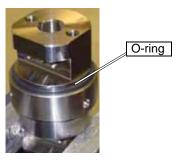
Figure B-27: Replace the O-ring with New One
