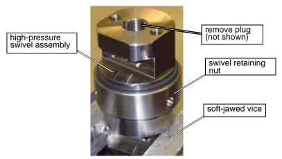
Figure B-4: Clamp the Swivel Assembly in a Soft-jawed Vice
