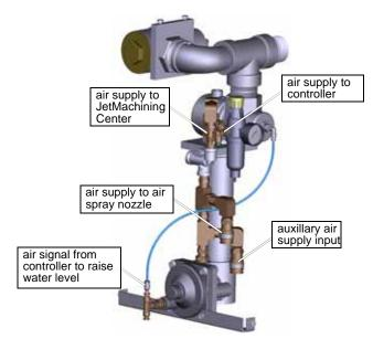
Figure 2-27: Rapid Water Level Control Internal Pneumatic Connections
