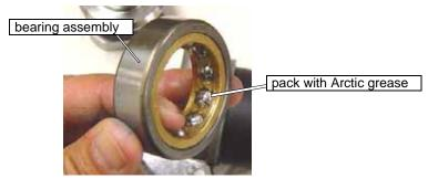
Figure B-18: Pack the Bearing Assembly with Arctic Grease
