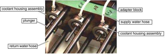
Figure 7-42: Coolant Housing Assembly Installation and Hose Connections
