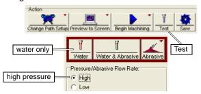
Figure C-20: Flushing the System with Water Only at High Pressure
