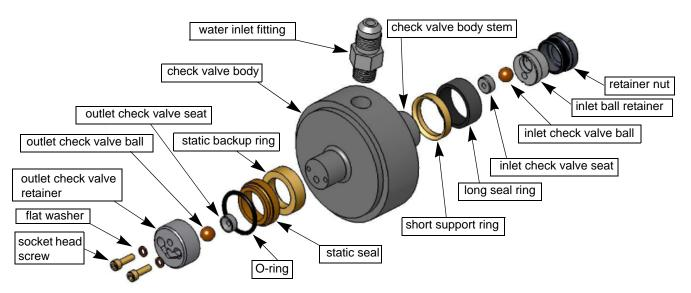
Figure 7-19: Check Valve Assembly Components
