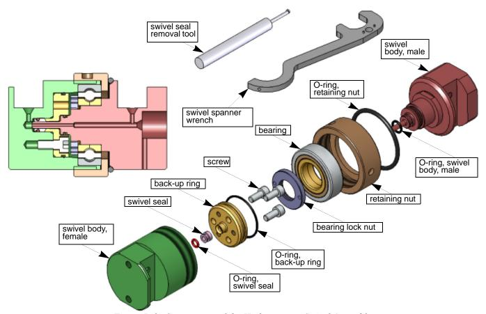
*Figure B-3: Components of the High-pressure Swivel Assembly*
