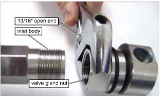
Figure C-5: Removing the Valve Gland Nut from the Nozzle Assembly
