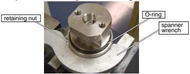
Figure B-26: Tightening the Retaining Nut with the Spanner Wrench
