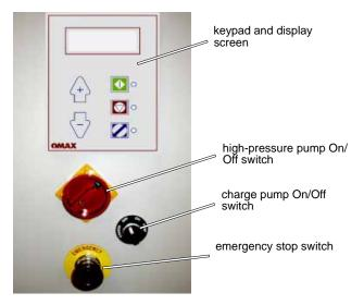
Figure 3-7: Pump Control Panel
