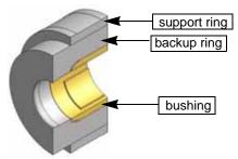
Figure 7-15: Backup Support Ring Assembly Components
