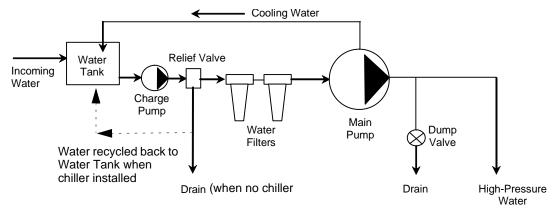
Figure 3-9: The Charge Pump Low-pressure Water Circuit
