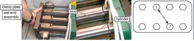
Figure 7-47: Installing the Clamp Plate
