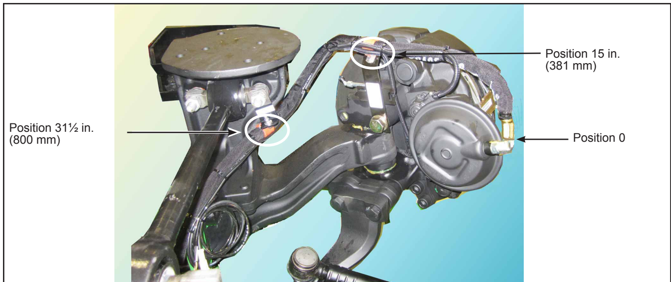
Figure 3 - P-Clamp Location on Hose
