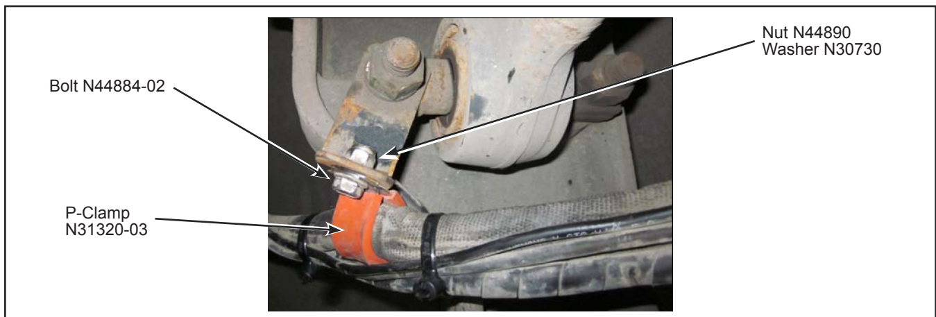
Figure 8 - L Support and P-Clamp Installation
