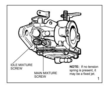
Start the engine and let it warm up for approximately 3-5 minutes. Do not adjust the carburetor when the engine is cold.
