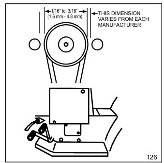
For proper declutching to occur, it is very important that the engine belt guide be set at a predetermined gap (set by the manufacturer) and away from the belt with the belt engaged.
