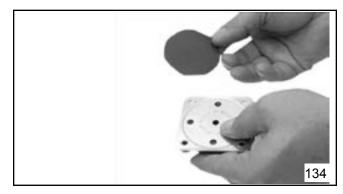
When reusing the old cover it is difficult to seal all five holes. One other way to compress the bellows is to invert the inside tab and place a slip knot made from thin string over it. Push the end of the bellows back to its original form and pull the string through the cover. When step six is complete, cut the string.
