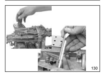
If the measurement is beyond the dimensions listed, the next step is to remove the transaxle from the frame. Then thoroughly wash and blow dry the bellows cover area as shown. Remove all impurities before removing the bellows cover.
