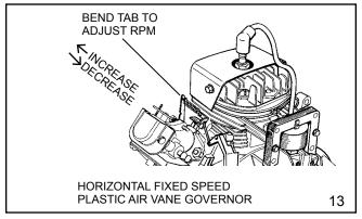
To disassemble, remove choke shutter with needlenose pliers; the vane assembly may then be removed from the carburetor.
