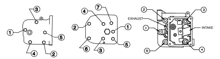
OVRM40-60, OHH, OHSK50-70 Torque bolts in 60 in. lb. (7 Nm) increments.
