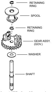
\* As of August 1992, all small frame engines, including VLV40-6.75, use a retainerless shaft. Service replacement shafts will be retainerless for all small frame and VLV engines.
