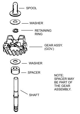
**NOTE:** On models OHV13.5-17, the spacer is cast as part of the governor gear with the washer placed below the gear assembly.
