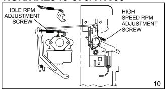
The HXL840 - 870 Series with variable speed control have the following adjustments. Idle speed is set at the carburetor crack screw. High speed is set with the screw shown above. Always check Microfiche card 30 or Parts Manager Pro computer program for correct speed settings.
