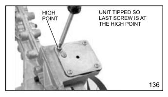
7. Remove the tape or cut the string allowing the bellows to expand into the oil. This expansion into the oil will push out most of the air from the chamber. When oil comes out from the loose screw tighten it and all other screws in a "X" pattern to a torque of 18-30 inch lbs. (2-3Nm). The unit is ready for installation.
