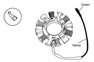
Yellow - Alternator A.C. Leads Red - Alternator D.C. (+) Leads Brown - Alternator D.C. (-) Leads
