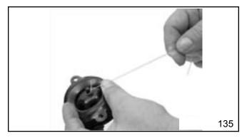
Install the bellows snugging down three of the four screws, DO NOT tighten them completely. Install the fourth screw a few threads then tip the unit slightly so the highest point is at the loose screw.
