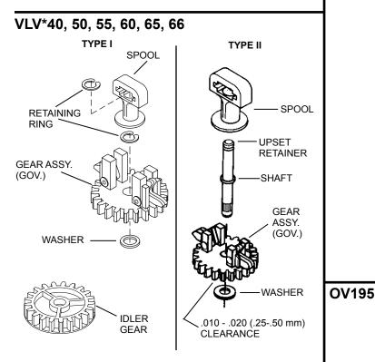
**NOTE:** Gear assembly must have .010 - .020 (.25 - .50 mm) end play after shaft is installed into flange.
