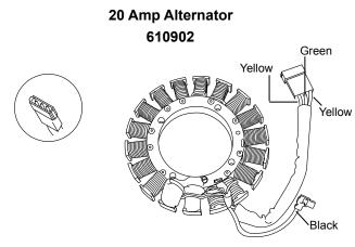
Uses regulator/rectifier 610996 or 610907A; depending on spec. number; an open circuit D.C. voltage check cannot be made.
