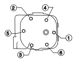
OHV11-17, OH120-180, OHM, OHSK, OVM, OVXL Torque bolts in 60 in. lb. (7 Nm) increments.
