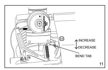
R.P.M. adjustment of fixed speed models is done by bending the tab as shown.
