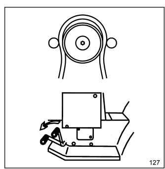
With clutch disengaged, it is very important that the belt blossoms away from the engine pulley. Belt must stop turning before transaxle shifting can occur.
