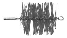
Plastic Brushes are recommended for removing soft deposits in straight ferrous and non ferrous tubes. Brush should be equal to the tube I.D.
