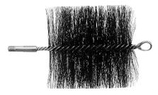
Carbon Steel Brushes are recommended for removing soft and light scale deposits in straight, ferrous tubes. Brush should be equal to the tube. I.D. (not recommended for stainless steel tubes).
