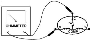
**TESTING COMPRESSOR WINDINGS**
