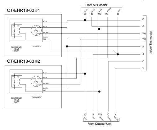
Typical Wiring Schematics for OT/EHR18-60 (Outdoor Thermostat & Emergency Heat Relay).
