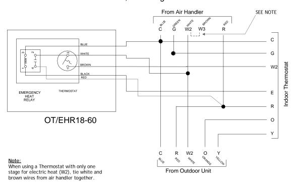
Typical Wiring Schematics for OT/EHR18-60 (Outdoor Thermostat & Emergency Heat Relay).
