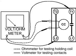
TESTING COMPRESSOR CONTACTOR
