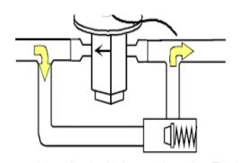
Most expansion valves used in current Amana® Brand Heat Pump products use an internally checked expansion valve.
