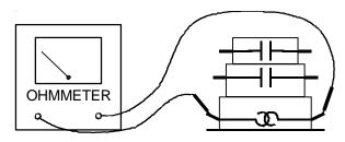
**TESTING COIL CIRCUIT**
