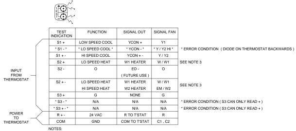
1.) THE TEST SPADE CAN BE CONNECTED TO ANY OTHER TEST SPADE ON EITHER BOARD.
