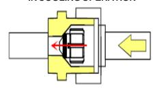
In the cooling mode, the orifice is pushed into its seat, forcing refrigerant to flow through the metered hole in the center of the orifice.
