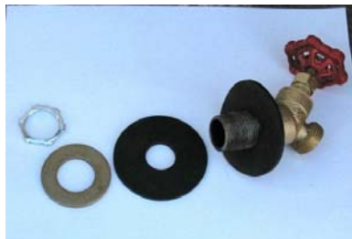
Parts for installing spigot, from left to right: a nut with pipe threads, metal washer, neoprene washer, 1-inch nipple, 2 nd neoprene washer placed on nipple, spigot (with nipple already attached).
