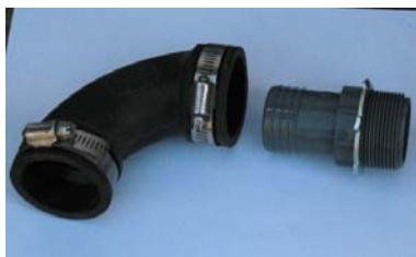
The overflow pipe is attached to the barrel using the plastic barbed adaptor (on the right) and the rubber elbow (on the left).
