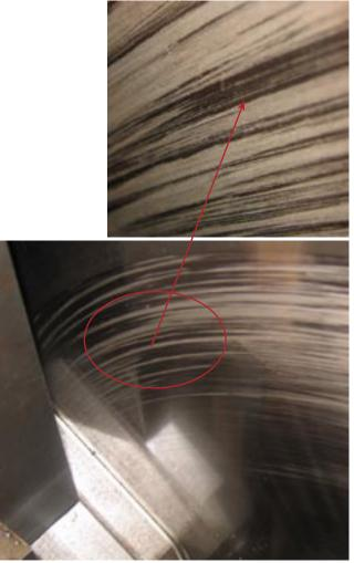
The greyish stripes on this thrust collar face indicate spark erosion
