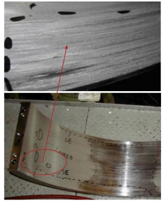
Corresponding lower bearing shell. Visible spark erosion, but no or limited wear can be measured.
