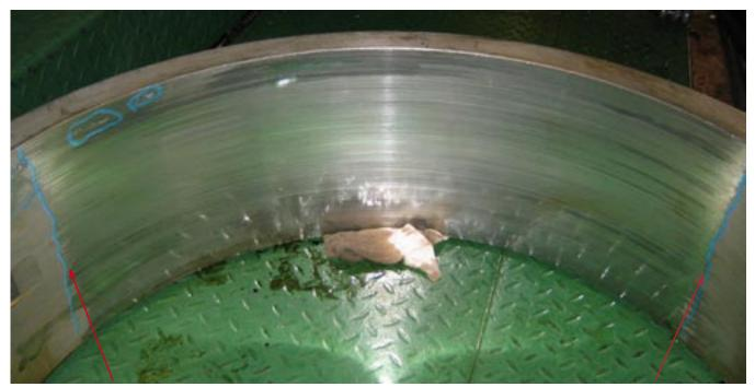
Corresponding main bearing lower shell with wide spread journal imprint. 0.5 mm of the shell is worn off between the two distinct, visible lines.
