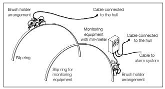
Shaftline earthing device parts
