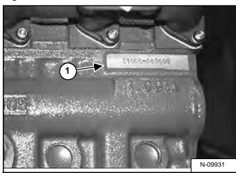
The engine serial number (Item 1) [Figure 3] is in the location shown.
