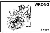
Lead-acid batteries produce flammable and explosive gases.
