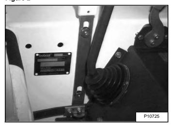
The loader serial number plate is located on the outside of the loader frame [Figure 2].
