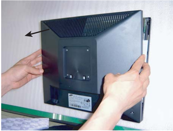
2. Lift up the back cover and Use the jig to remove the shield lamp.
