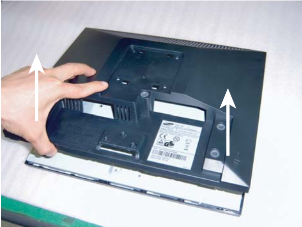
3. Lift up the back cover and Use the jig to remove the shield lamp.
