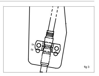
3. The cable is clamped using the top set of holes on the hanger plate. These are marked 40 on the surface of the hanger plate. (fig 3).
