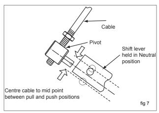
11. Insert pivot (9) into shift lever (3) and fit split pin (10) do not spread split pin at this stage. Ensure that the attachment pin of the pivot does not bind in the shift lever hole.
