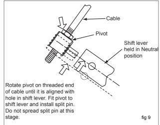
Verify by pulling and pushing cable to establish mid point of travel. The pivot pin should be re aligned with hole in shift lever.
