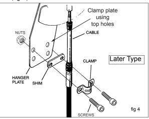
During assembly ensure that the protrusion on the inside face of the clamp is correctly located in the recess on the cable ferrule. Ensure that a new cable clamp, shim and fixings are used.
