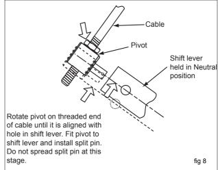
Move range selector through all positions to ensure that it is synchronised with the transmission. Adjust pivot if necessary, spread split pin and tighten rod nut against pivot.
