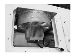
e) Remove fan diffuser and replace fan motor.(The screw of fan fixing nut (M14) is reverse direction.)
