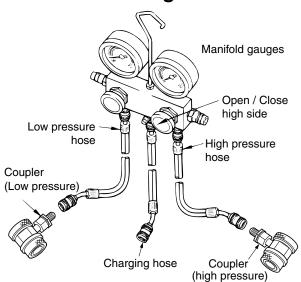
Structure of manifold gauges
