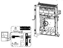
Fig.1 Layout of inverter boards TP1 and TP2
