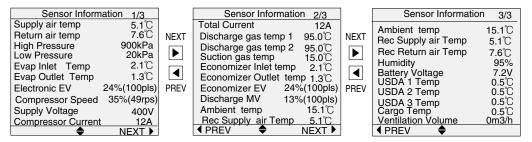
Notes 1. "ERROR" is displayed in the case of sensor failure.
