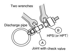
Fig. 1 Use two wrenches when removing and installing.
