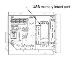
USB memory connected to the controller
