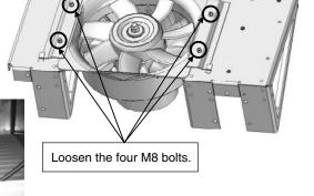
d) Pull the fan assembly straight out.
