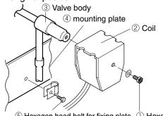
⑤ Hexagon head bolt for fixing plate ① Hexagon head bolt
