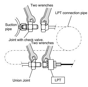
Fig. 5 Use two wrenches for loosening and tightening flare nuts
