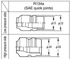
Be sure to use the manifold gauges with the quick joints shown above.
