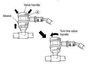
Note: Do not fully turn the valve handle clockwise. Otherwise, the push pin may be broken.
