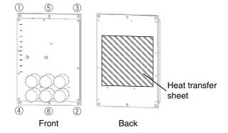
Fig.3 Inverter board
