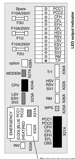
Short circuit connectors for emergency operation
