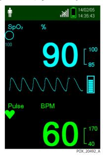
**Figure 4-36.** %SpO<sub>2</sub> of 90 with High Modulation
