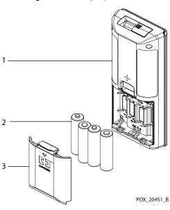
Figure 6-3. Battery Replacement
