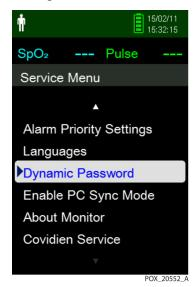
4. Highlight the mode transition for which the password is being changed, then press OK.
