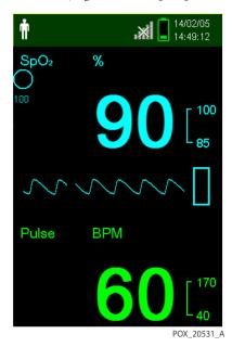
**Figure 4-42.** %SpO<sub>2</sub> of 90 with High Light Condition
