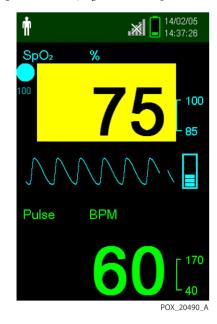
**Figure 4-37.** %SpO<sub>2</sub> of 75 with High Modulation
