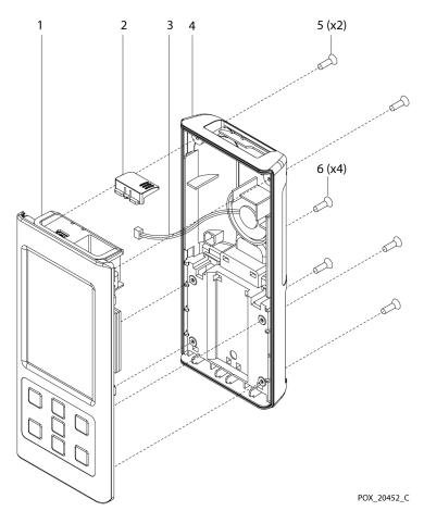
Figure 6-4. Front and Rear Assembly Replacement
