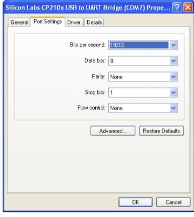
Figure 3-10. Baud Rate List, Port Settings Tab
