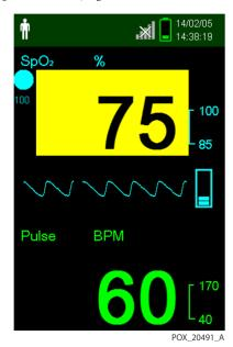
**Figure 4-38.** %SpO<sub>2</sub> of 75 with Low Modulation
