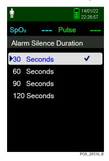
Figure 4-14. Alarm Silence Duration Setting of 30 Seconds
