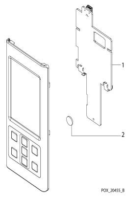
Figure 6-7. Coin Cell Battery Replacement
