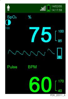
Figure 4-28. SRC-MAX Tester-Generated Waveform
