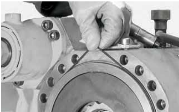
FIGURE 22: Check quality and position of the cylinder's o-ring.
