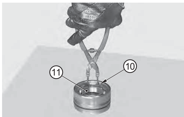
FIGURE 7: Fit the snap ring (10) on the bearing (11).
