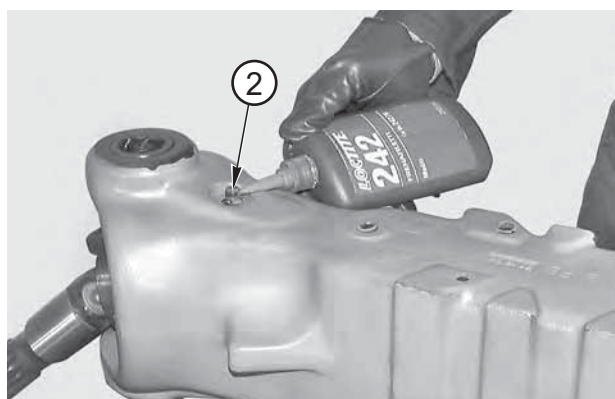
FIGURE 11: Apply Loctite 242 to the jutting parts of the studs (2).
