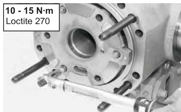
FIGURE 31: Apply LOCTITE 270 to the thread of the piston adjustment nut. Tighten with torque wrench setting of 10 - 15 N·m
