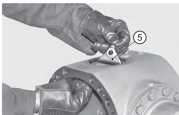
FIGURE 9: Extract selector fork (5).
