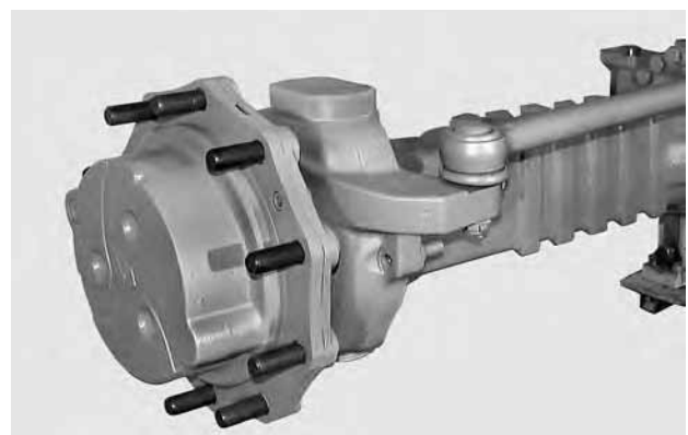
FIGURE 40: Connect the steering bars. For details, see COMPLETE STEERING CASE p. 25.
