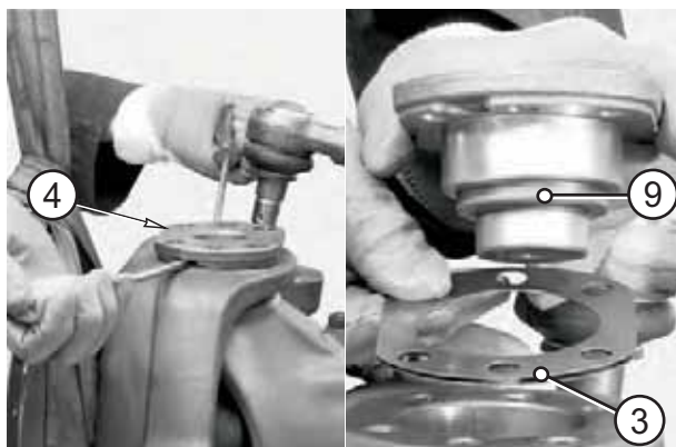
FIGURE 2: Using two levers, remove the top articulation pin (4) complete with front seal (9) and shims (3).
