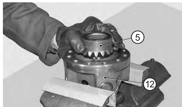
FIGURE 23: Position the second planetary gear (6) in the differential carrier (12).
