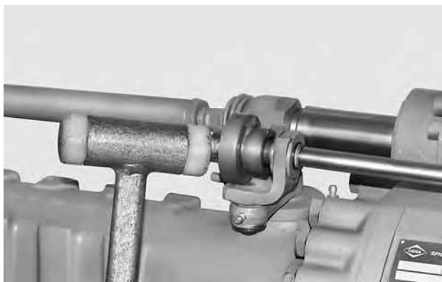
FIGURE 1: Before starting any operation on the assembly, disable the cylinder by giving a light hammer blow to the external ring of the check unit.
