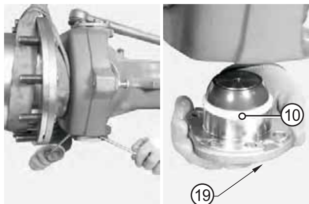
FIGURE 3: Remove the bottom articulation (19) pin complete with front sealing ring (10).
