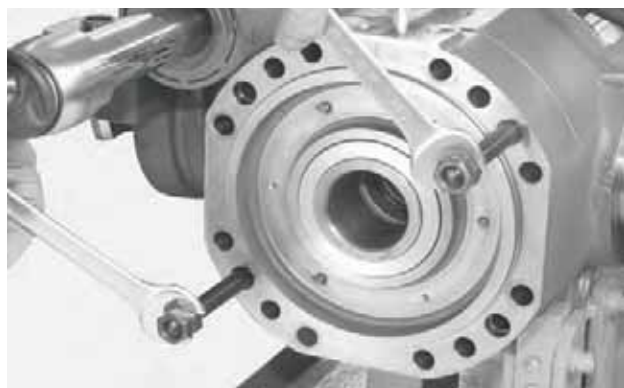
FIGURE 8: Loosen the studs and remove two of them.
