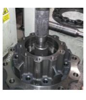
IMPORTANT: check the force exerted by the press to remove the bearing cup. If the force is lower than 10kN [1ton=1000kgf], the hub can NOT be reused, it must be discarded and replaced by a new complete hub & bearing assembly.
