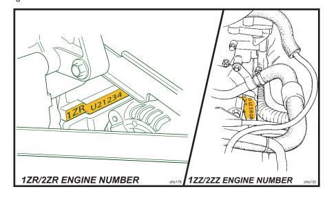
1ZZ and 2ZZ engine numbers are marked on a vertical patch at the right hand side of the rear face of the cylinder block, adjacent to the clutch housing.
