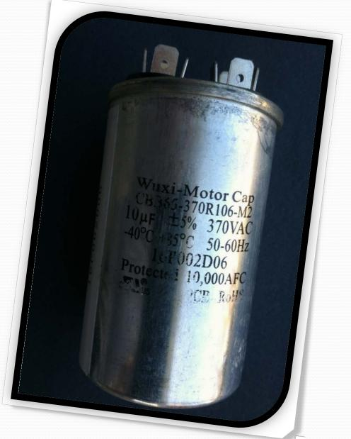
This can be accomplished by removing the fan wires from the top and touching a screw driver across the top and to the back of the control box. Once the voltage has leaked then you can either test for micro fahrens with a MFD tester or replace the capacitor. 609-386-1012
