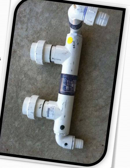
After everything is disconnected the best way to get the old manifold out of the machine is to cut it out with a rope saw, if your going to use a reciprocating saw be very careful not to hit the aluminum coil. When installing the new manifold you will notice that it is a very tight fit, slide the hoses onto the heat exchanger as far as possible create more room for installation.
