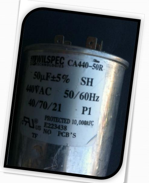
This can be accomplished by removing the compressor wires from the top and touching a screw driver across the top and to the back of the control box. Once the voltage has leaked then you can either test for micro fahrens with a MFD tester or replace the capacitor.
