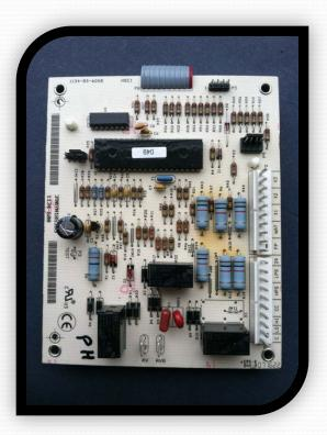
Then remove the four screw holding the board to the front of the control box. Finally reattach the new board and reconnect the three wire harnesses previously removed.
