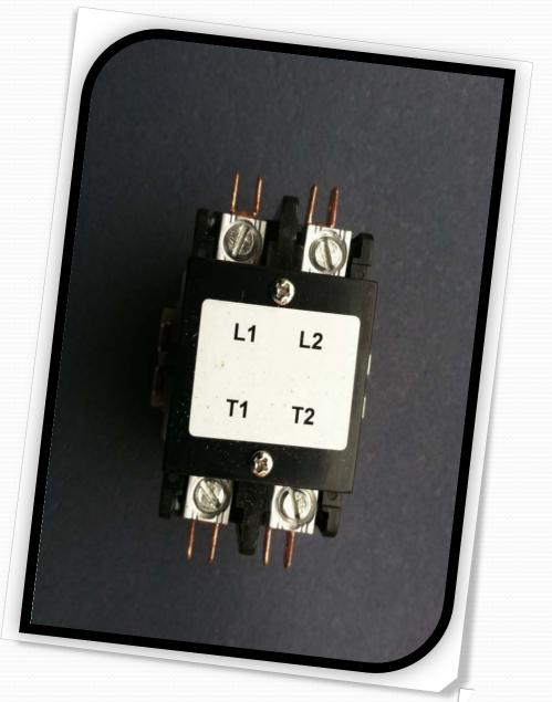
There are many wires on a contactor , when changing it out it is best to remove one at a time and connect them to the new piece so that they don't get mixed up. Then remove the old contactor from the control box and mount the new contactor.
