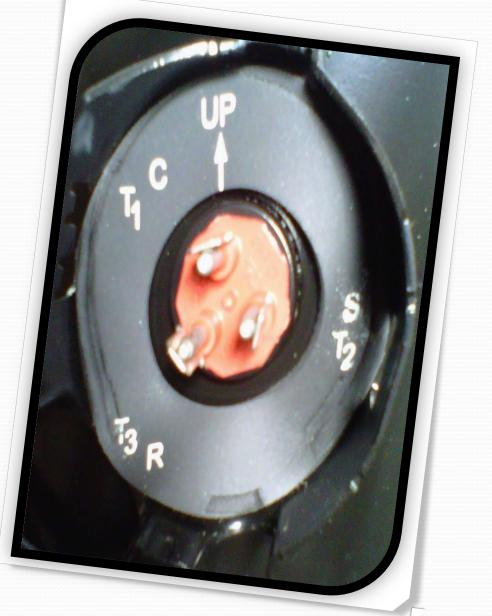
An additional indicator will be that the compressor will be very hot to the touch. The compressor will need time to cool down and the overload switch will have to close before the compressor will work.(you can not manually close the switch) If a test results in an open winding (OL) the compressor will not turn on.
