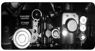
5400 filter housing cap. (do not over tighten)
