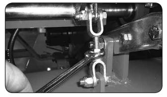
The deck spring tension is critical. If the tension is too much, it will cause the spring to break. If too loose, the belt can jump off or slip on the pulleys and cause a cut quality issue. With the deck up, the spring coil gap should be about .025" - .030" (about the thickness of a credit card). Spring tension adjustments can be made by sliding the bolt shown above forward or backward in the slot of the deck.
