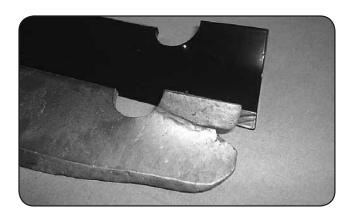
To change blades, it may be easier to use a piece of wood to keep the blade from turning so that the bolt can be loosened. Re-torque the blade bolts to 90-110 lbs. The blade spindles contain a sealed ball bearing in the top and bottom of the spindle. The bearings are replaceable for a more cost effective repair.
