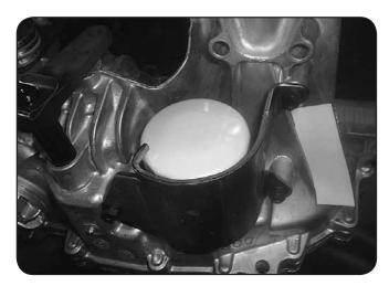
Shown right is the 5400 Outlaw transaxle. The large cap on the lower left is the filter housing cap.
