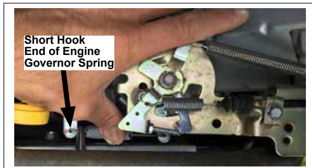
Figure 1. Disconnect Governor Spring.
