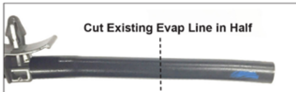
Figure 1. Cut Existing Evap Line in Half.
