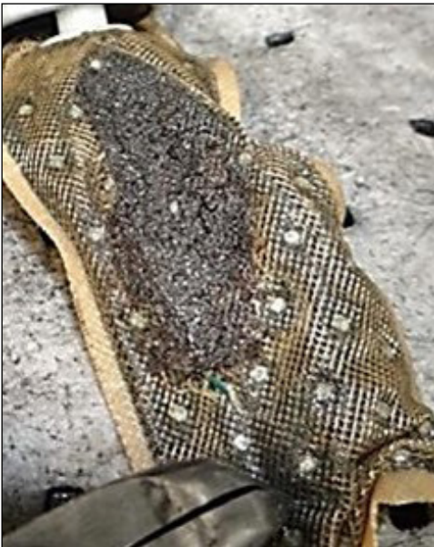
Filter Inside Fuel Pump Module when Incorrect Micron Fuel Filter is Used
