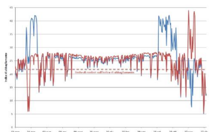
Numeric values of the glaring index – for one day on the left and for a full year on the right (the red dotted horizontal line refers to the upper limit of comfort conditions)
