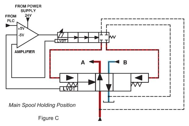
Many external amplifiers have a "Broken Wire" light that will come on if there is no signal from the main spool LVDT. If the light flickers, this means there is a loose connection. To check the proportional valve, there are two electrical tests that can be made. The hydraulic supply should be off and any pressurized fluid in the accumulator should be dumped to tank. Specific instructions and terminals for your exact amplifier should be referenced.
