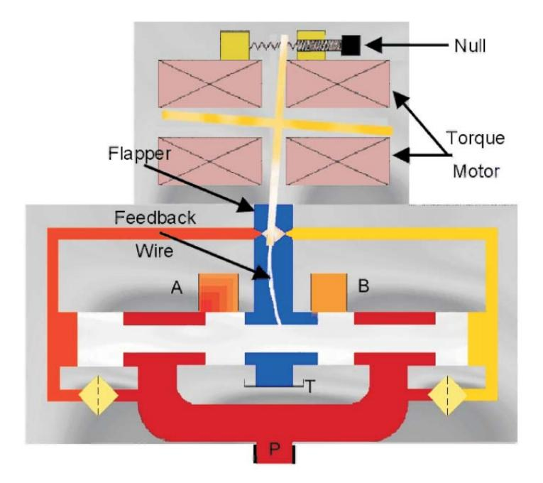
When a current signal is applied to the valve coil, the torque motor rotates, moving the flapper closer to the left nozzle. Pilot pressure builds up on the left side of the main spool. The valve spool shifts, connecting the P to A ports and the B to T ports. As the spool shifts, the feedback wire bends.
