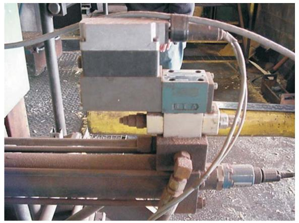
Hydraulic Cylinder with a Temposonic Transducer
