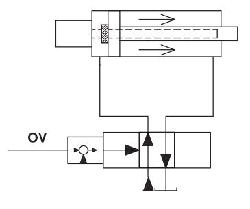
The system should be at normal temperature when nulling the valve. To null the valve, the electrics should first be disconnected. Remove the null access screw to get to the allen head null adjustment. On some servos the null adjustment is located on the main spool.
