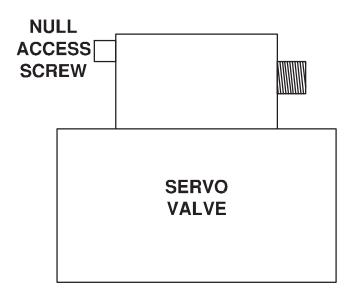
The null is usually a 1/8" or 3/16" allen head. If possible use a brass wrench as it won't interfere with the magnetism in the coils. Observe the cylinder drift while nulling. The adjustment should not be turned more than 1 or 2 turns maximum. When the cylinder stops drifting, the valve is nulled.
