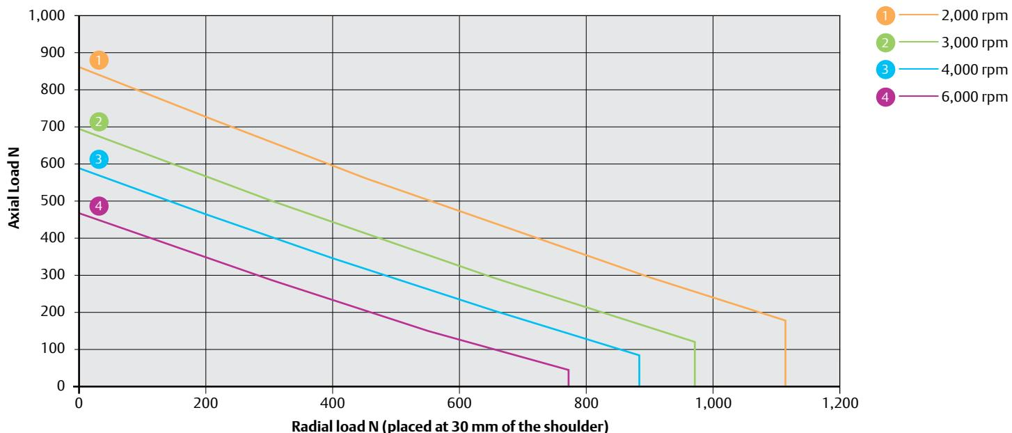
115UD/ED  $L_{10(h)}$  Bearing life for 20,000 hours (reliability 90 %, load factor of 1). Do not exceed a maximum axial load of 1,200 N
