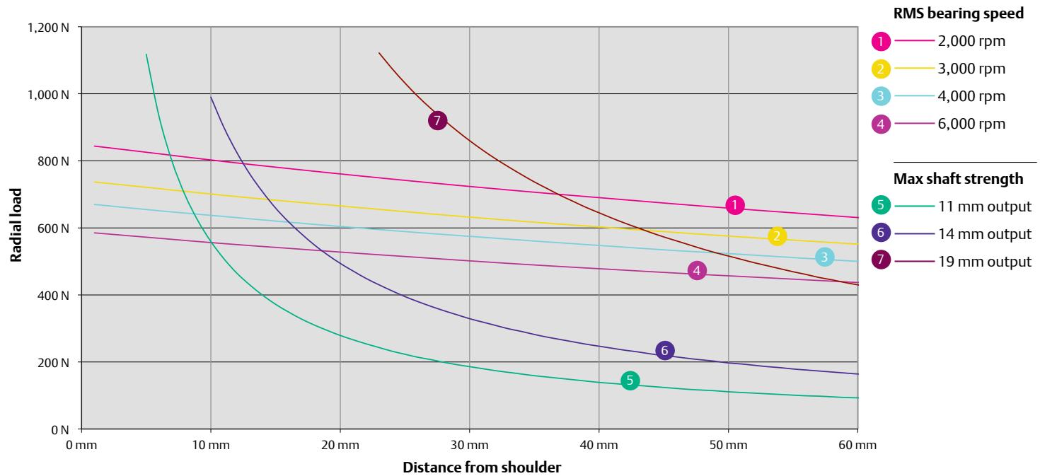
75U3/E3 L<sub>10(h)</sub> Bearing life and output shaft strength (20,000 hours, 90% reliability, load factor of 1)
