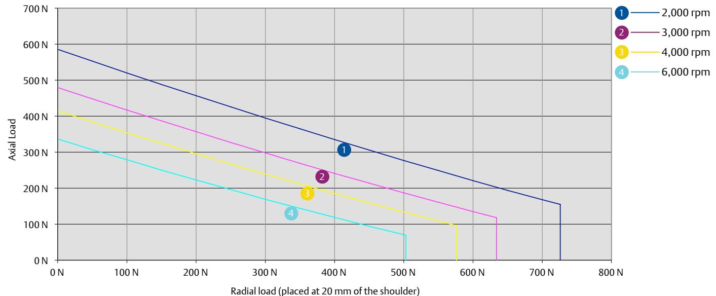
75U3/E3 L<sub>10(h)</sub> Bearing life for 20,000 hours (reliability 90 %, load factor of 1). Do not exceed a maximum axial load of 900 N
