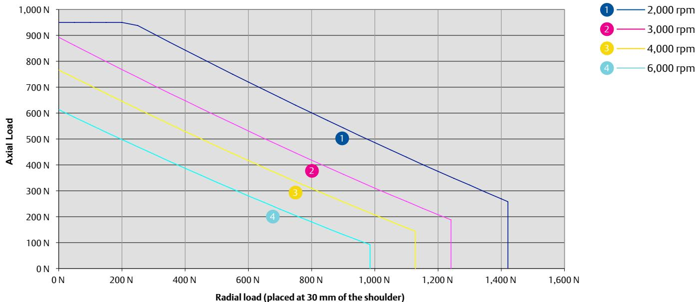
142U3/E3  $L_{10(h)}$  Bearing life for 20,000 hours (reliability 90 %, load factor of 1). Do not exceed a maximum axial load of 950 N
