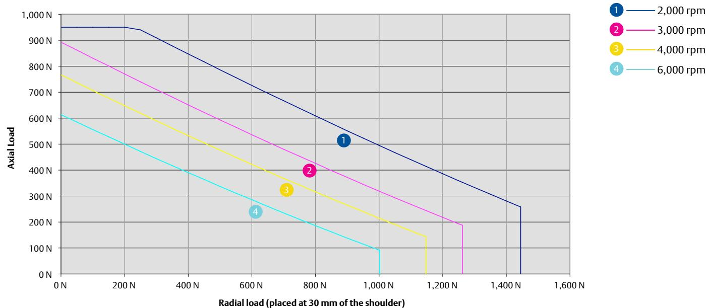
115U3/E3 L<sub>10(h)</sub> Bearing life for 20,000 hours (reliability 90 %, load factor of 1). Do not exceed a maximum axial load of 950 N
