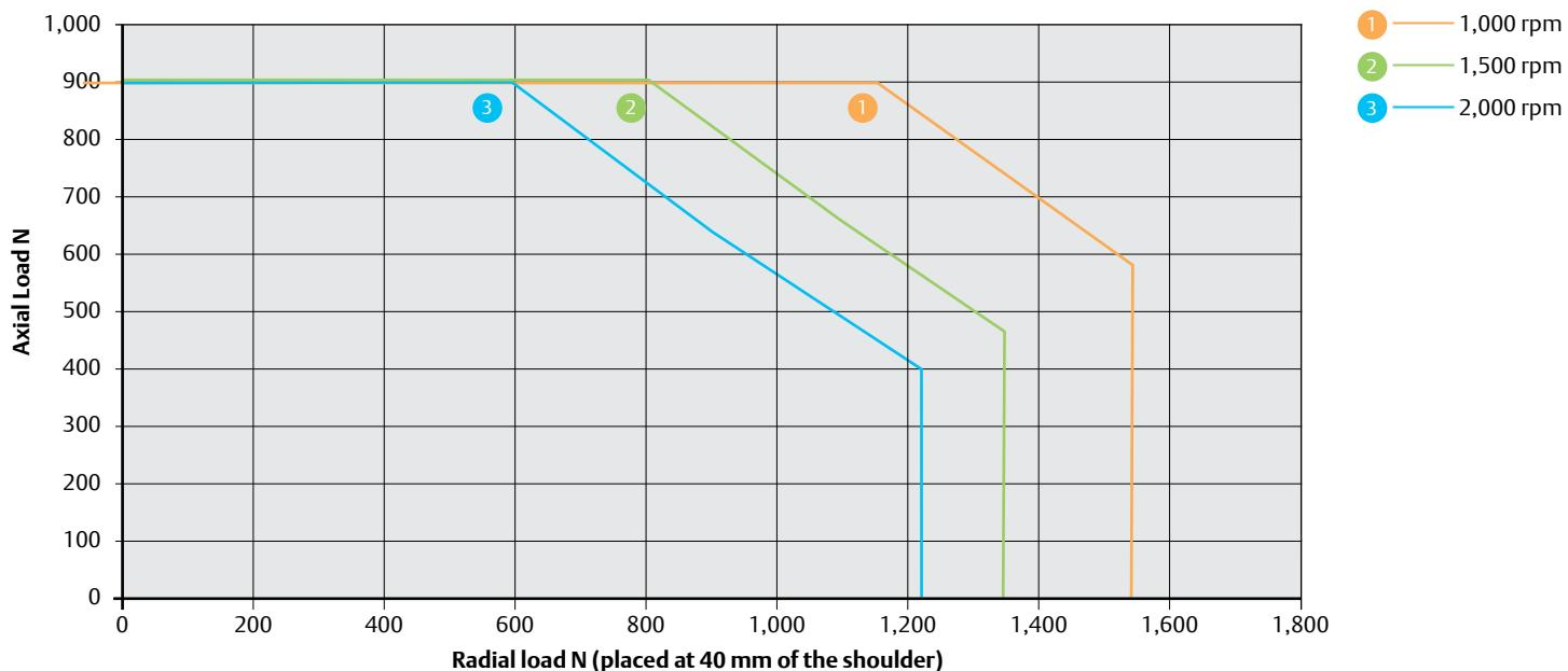
190UD/ED  $L_{10(h)}$  Bearing life for 20,000 hours (reliability 90 %, load factor of 1). Do not exceed a maximum axial load of 900 N
