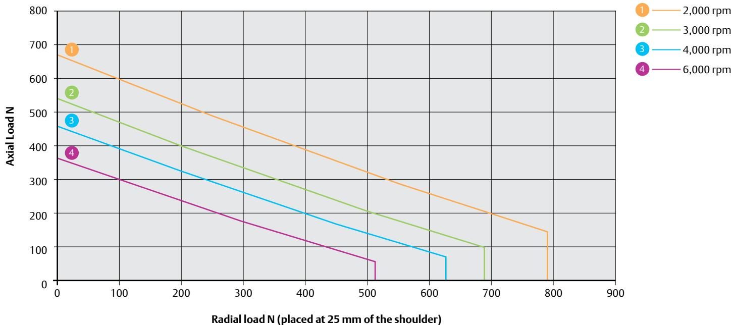
089UD/ED  $L_{10(h)}$  Bearing life for 20,000 hours (reliability 90 %, load factor of 1). Do not exceed a maximum axial load of 1,000 N
