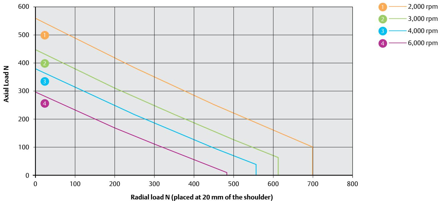
067UD/ED  $L_{10(h)}$  Bearing life for 20,000 hours (reliability 90 %, load factor of 1). Do not exceed a maximum axial load of 650 N
