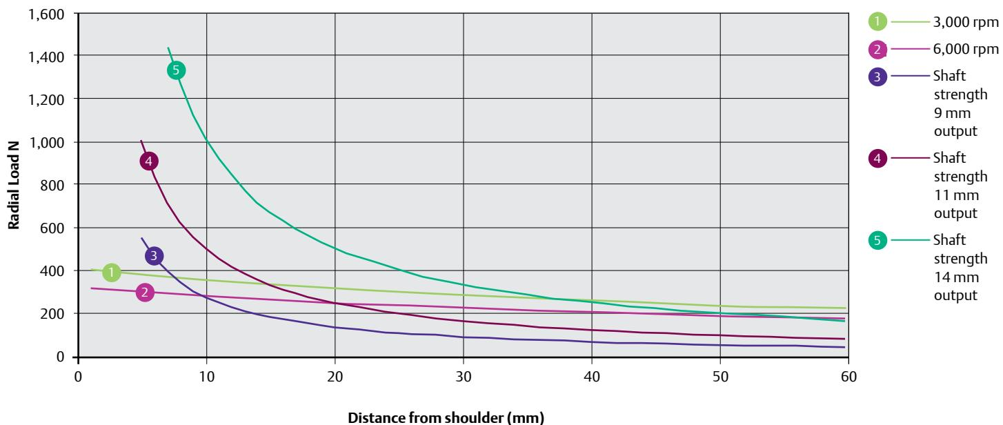
055UD/ED  $L_{10(h)}$  Bearing life for 20,000 hours (reliability 90 %, load factor of 1). Do not exceed a maximum axial load of 450 N
