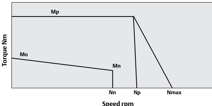
Mn = continuous torque at the rated speed: Nn = rated speed:
