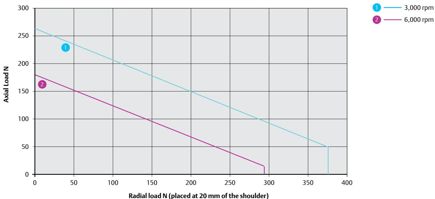
055UD/ED  $L_{10(h)}$  Bearing life for 20,000 hours (reliability 90 %, load factor of 1). Do not exceed a maximum axial load of 650 N
