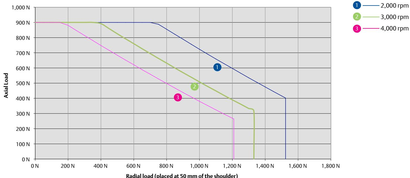
190U3/E3  $L_{10(h)}$  Bearing life for 20,000 hours (reliability 90 %, load factor of 1). Do not exceed a maximum axial load of 900 N
