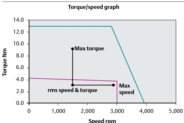
Max torque = 10 Nm: Max speed = 2,900 rms torque = 3 Nm: rms speed = 1,500
