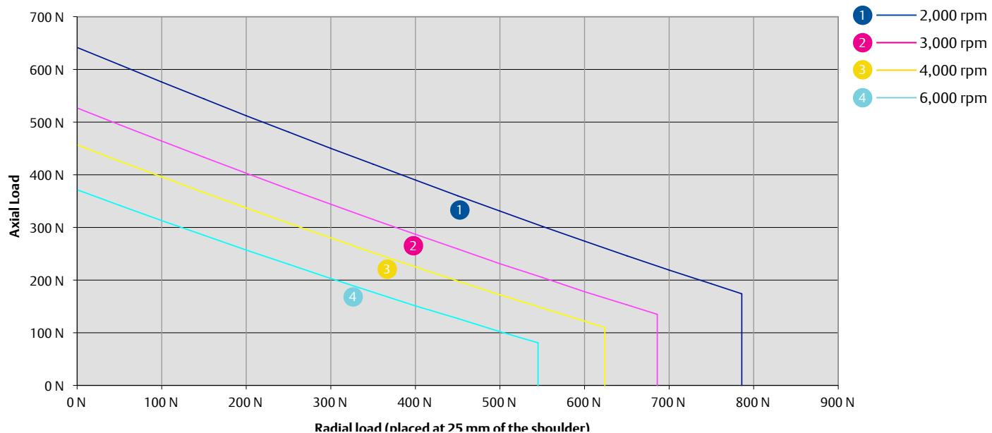
95U3/E3 L<sub>10(h)</sub> Bearing life for 20,000 hours (reliability 90 %, load factor of 1). Do not exceed a maximum axial load of 850 N
