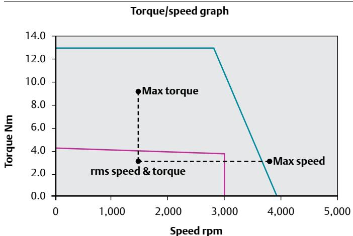
Max torque = 10 Nm: Max speed = 3,900 rms torque = 3 Nm: rms speed = 1,500
