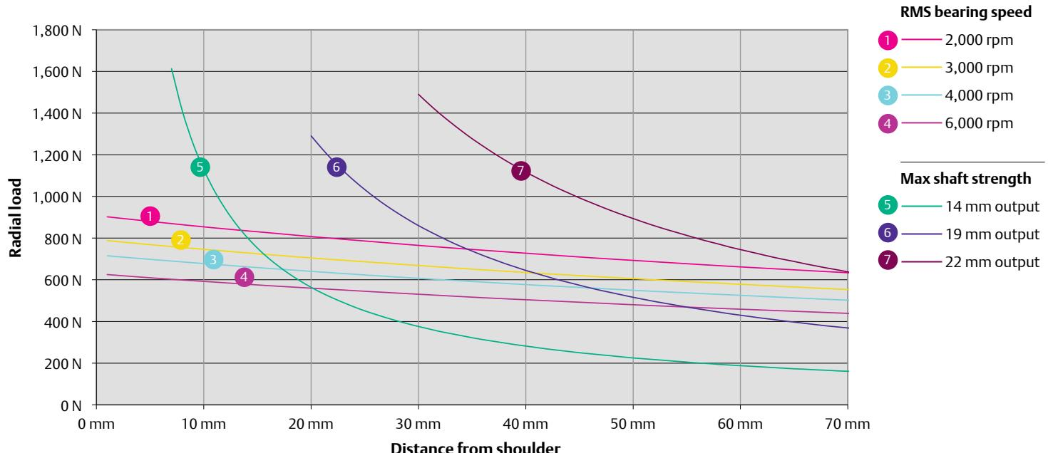
95U3/E3 L<sub>10(h)</sub> Bearing life and output shaft strength (20,000 hours, 90% reliability, load factor of 1)
