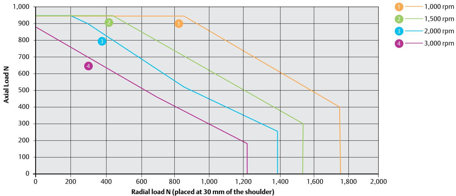
142UD/ED  $L_{10(h)}$  Bearing life for 20,000 hours (reliability 90 %, load factor of 1). Do not exceed a maximum axial load of 950 N
