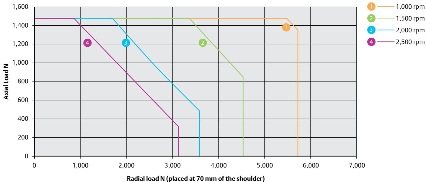
250U3 L<sub>10(h)</sub> Bearing life for 20,000 hours (reliability 90 %, load factor of 1). Do not exceed a maximum axial load of 1,450 N
