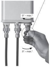
Set downtilt angle by rotating the gearwheel.
