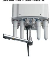
Carefully place the connector and fix the nut using a torque-wrench (according to the manufacturers guidelines).
