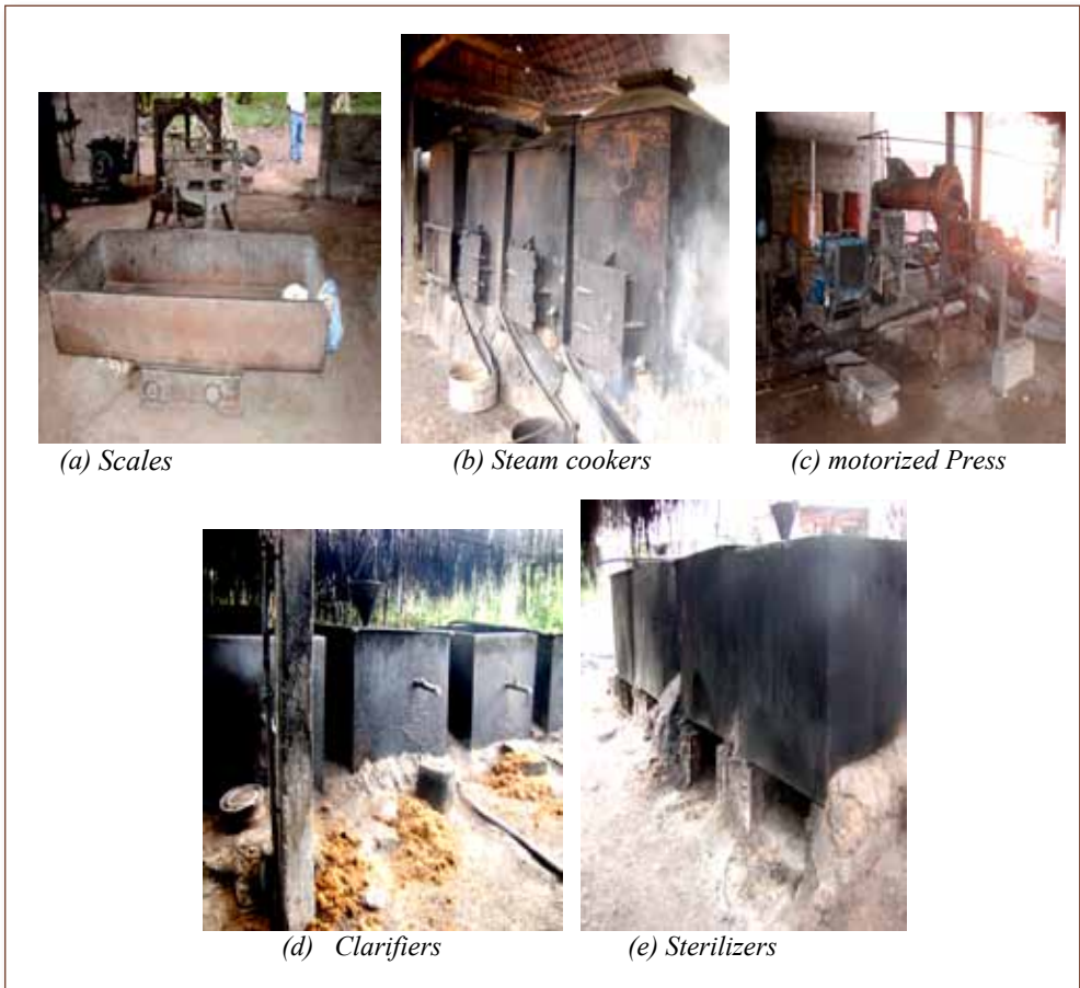
Fig. 4.20a-e. Palm fruit processing: a) scales for weighing fruit, b) steam cooker, c) motorised press, d) clarifiers, e) sterilisers (Photos from J. Hounhouigan)
