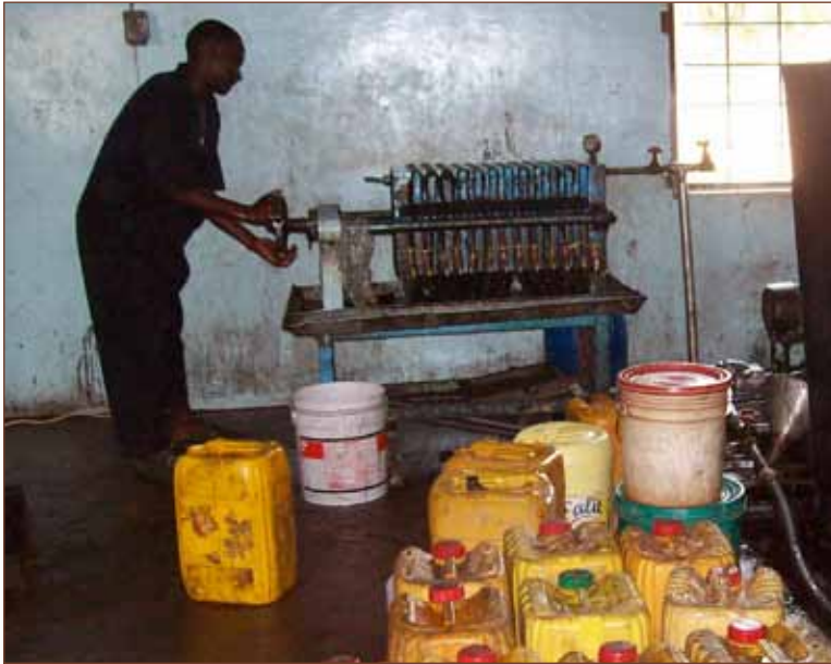
Fig 4.8. Plate and frame filter press for clarifying oil (Photo from L. Gedi)
