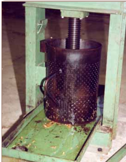
Fig. 4.4. Screw press (a) from Practical Action Publishing, (b) (Photo from P. Fellows)
