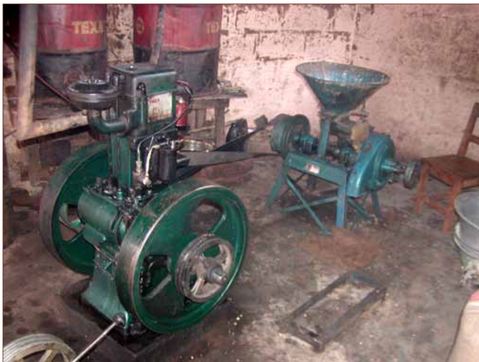
Fig 4.16. Diesel powered mill for grinding groundnuts for small-scale production (Photo from J. Hounhouigan)
