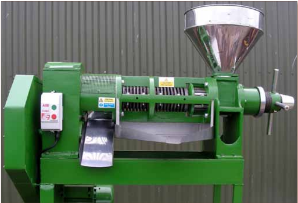
Fig 4.6. Small/medium scale oil expeller with capacities up to 150 kg seed/hr (Photo from Alan Brewis)
