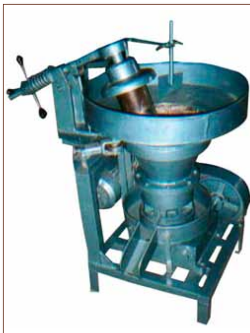
Fig. 4.3. Ghani used for oil extraction (Photo from Tiny Tech Plants (pvt) Ltd.)
