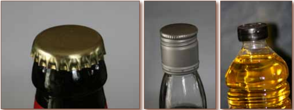
Fig 3.12. Caps for sealing bottles: a) Crown cap, b) metal roll-on-pilfer-proof (ROPP) cap, c) plastic ROPP cap (Photos from P. Fellows)
