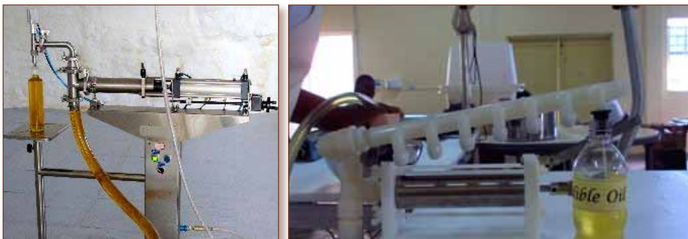
Fig 3.9a). Dispenser for filling oil - range 100 - 1000 ml, typically 600 bottles/hour. (Photo from Alan Brewis), b) Manual filler for filling up to seven bottles - the lever on the right moves the piston, centre (Photo from Franklin Murphy)
