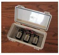
a butter knife, placed between the terminals at the top of the battery. Twist the knife to move the battery away from the battery holder. Then take the knife and place it at the bottom of the battery inside the battery holder. Pry the battery up and out of the holder to discard.
