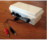
take the two colored alligator clips and apply them to the ends of the silver rods visible above the surface of the Silva-Cap. It does not matter which colored clip attaches to which rod. Note: This is all the action needed to set the generator to work! A low voltage circuit is created between the positive and negative battery poles by the rods inside the distilled water. You have now begun the process of production.
