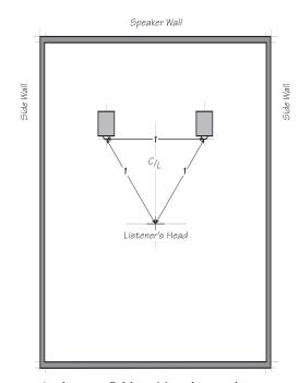
In the near field position the speakers and the listener's head are the points of an equilateral triangle. Near field listening gives the perfect stereo field. It is frequently used in the recording studio to position the microphones and the voice in the mix. The near field listening position is determined by the "center to center" distance of the speakers and the distance to the listener's head. It does not refer to the room in any way.
