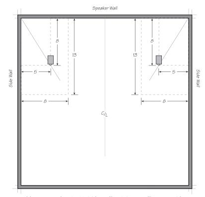
Golden Rectangles, 1.618 (side wall) x 1 (rear wall) on one side and 1 (side wall) x 1.618 (rear wall) create diagonal lines for speaker placement in a square room.
