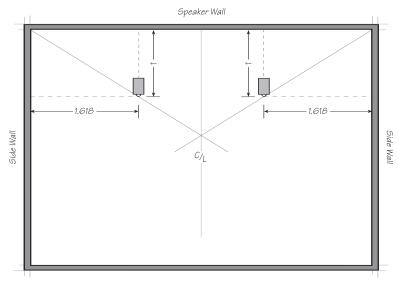
Golden Rectangles, 1.618 from the side walls x 1 from the rear wall, create diagonal lines for speaker placement in a horizontal room.
