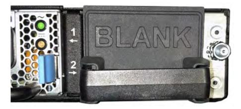
Figure 6: Chassis ground lug
