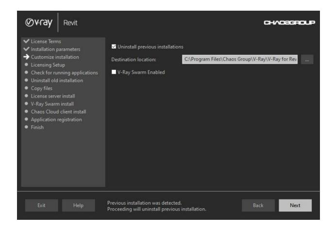
4. The next screen configures the Licensing Setup installation. The connection to the V-Ray license server by default is **Local V-Ray license server on this machine**. You can also choose to customize the installation.
