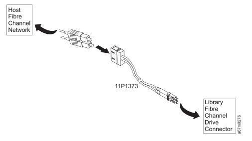
Figure 2-14. Interposer installation
