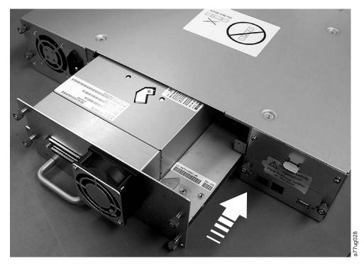
Figure 9-4. Pushing the drive into the library
