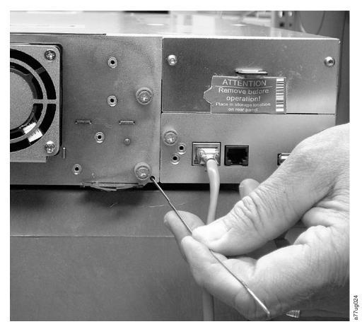
Figure 8-2. Access holes for the right magazine
