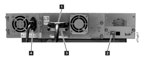
Figure 2-12. Attaching a SCSI host interface cable to the 2U library
