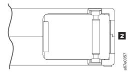
Figure 5-8. Leader pin in the incorrect and correct positions. The cartridge door is open and the leader pin is visible inside the cartridge.
