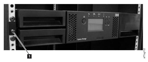
Figure 9-10. Removing the two screws anchoring the library to the rack
