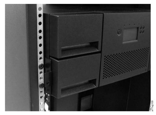
Figure 2-9. Sliding the 4U library into the rack
