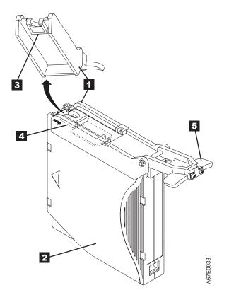
Figure 5-12. Attaching the leader pin attach tool to the cartridge. To hold the cartridge door open, hook the tool into the door and pull the tool back.
