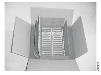
Figure 5-6. Double-boxing tape cartridges for shipping
