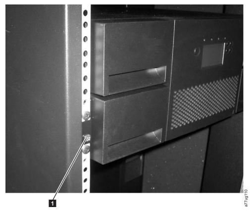
Figure 2-11. Securing the 4U library to the rack
