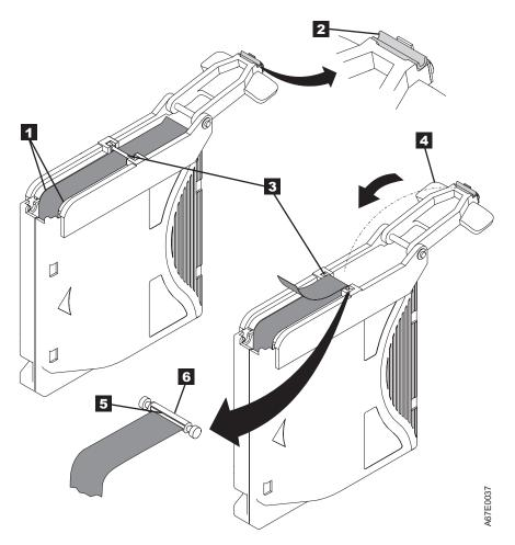
Figure 5-15. Attaching the leader pin to the tape
