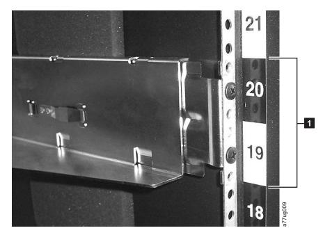
Figure 2-5. Rear view of a rail installed in a rack
