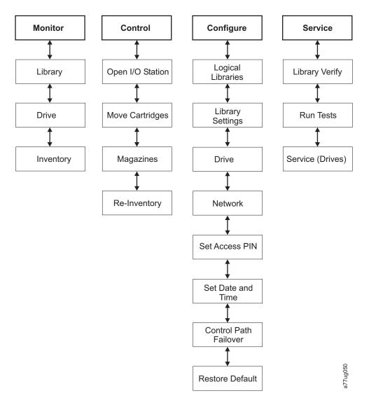
Figure 4-1. Operator Control Panel Menu Tree
