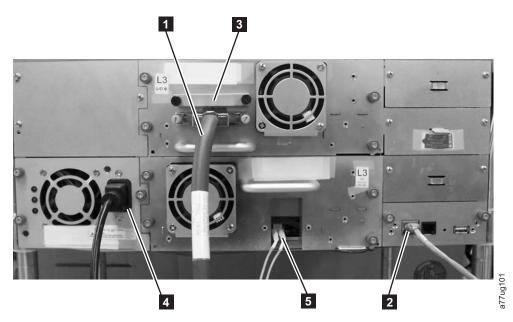
Figure 2-13. Attaching host interface cables to the 4U library. This 4U library contains one SCSI drive and one Fibre Channel drive.
