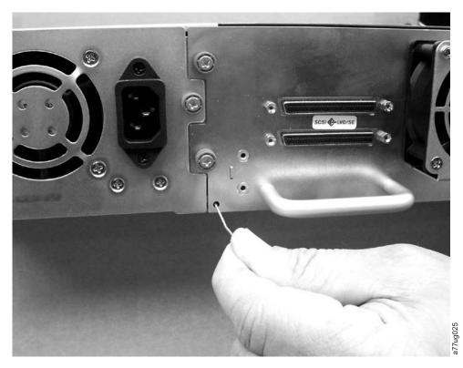
Figure 8-1. Access holes for the left magazine
