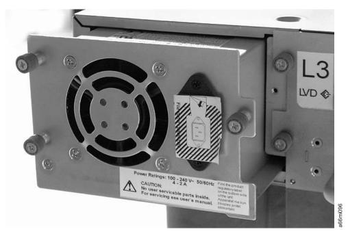
Figure 9-5. A power supply being removed from the library
