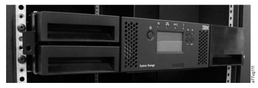
Figure 2-8. Sliding the 2U library into the rack
