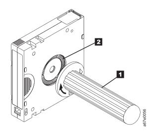
Figure 5-10. Rewinding the tape into the cartridge
