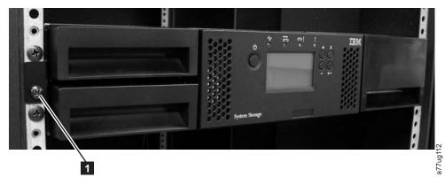
Figure 2-10. Securing the 2U library to the rack
