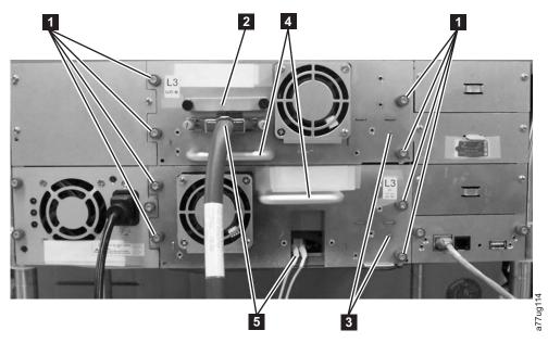
Figure 9-2. Drive Sled Components on back panel of 4U Library (SCSI and FC both shown)
