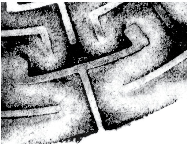
ACTUAL GASEOUS FLOW THROUGH RAVEN TRIM.
