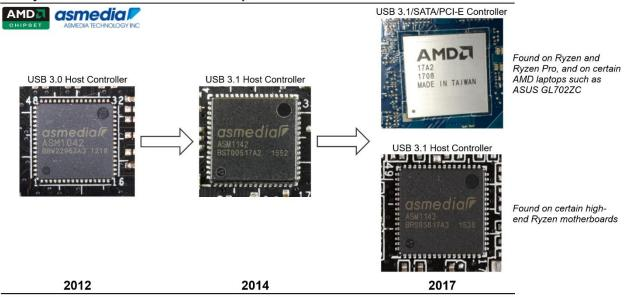
Our analysis suggests that *AMD Promontory* is heavily based on the design of *ASMedia ASM1142*. A comparison of the firmwares has shown that, during development, massive amounts of code were copied over from *ASM1142* into *AMD Promontory*, transferring many security vulnerabilities into AMD's *Ryzen* chipset.
