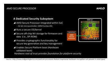
One of the primary functions of the *Secure Processor* is to act as the immutable *Root of Trust* for verifying the secure boot process. This feature allows for AMD's *Hardware Validated Boot*.
